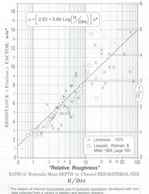
Figure D1: Resistance (Friction) Factor versus Ratio of Mean Depth to Bed Material Size
