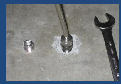
Purge sampling probe with vacuum pump before taking samples with either a syringe or canister.
