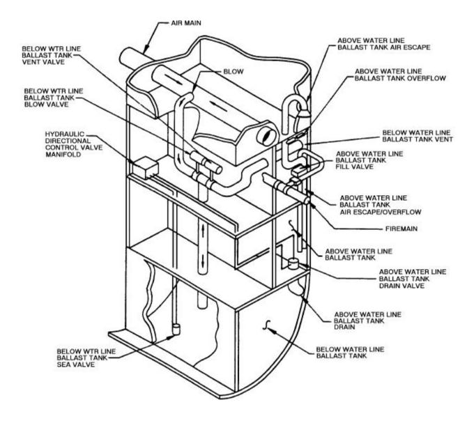
Figure 1. Typical Amphibious Ship Ballast and Deballast Tank Piping Composite
