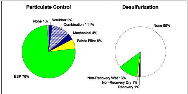
Figure 3-3. Air Pollution Control Technologies Used at Coal-Fired Utilities
