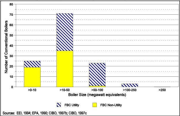
Figure 5-3. Capacities of Utility and Non-Utility FBC Units
