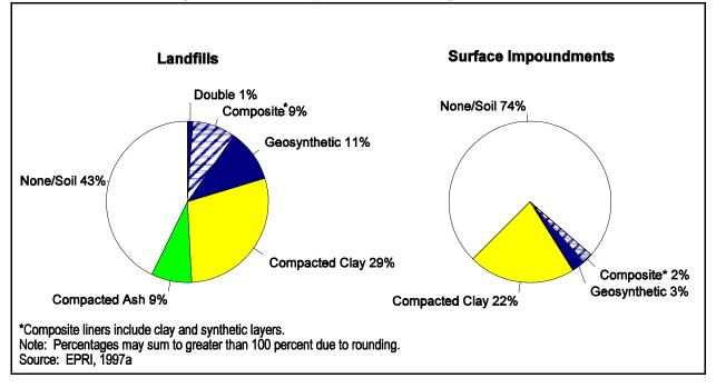
Figure 3-9. Liner Types for Comanagement Units
