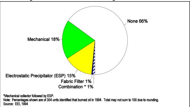
Figure 6-3. Particulate Control Technologies at Oil-Fired Utilities
