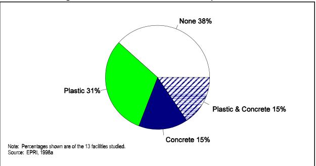
Figure 6-3. Liners Used in OCW Surface Impoundments
