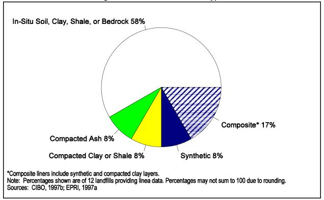
Figure 5-5. FBC Landfill Liner Types
