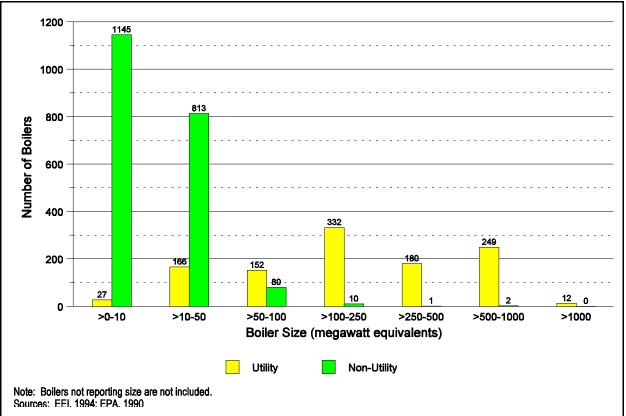
Figure 4-4. Distribution of Coal-Fired Boilers by Capacity
