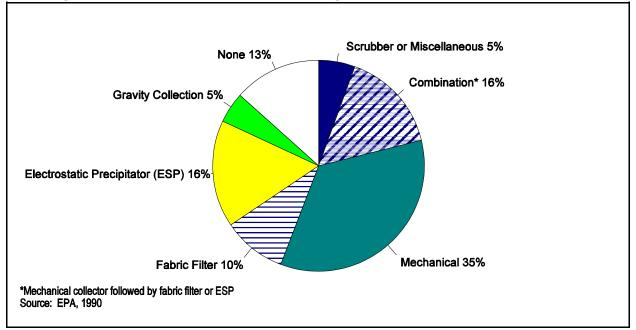
Figure 4-5. Particulate Control Technologies Used at Coal-Fired Non-Utilities
