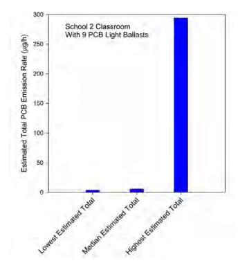
Figure 4-2. Example of the estimated range of total PCB emission rates from fluorescent light ballasts in a school classroom using the lowest, median, and highest rates from chamber tests of four ballasts
