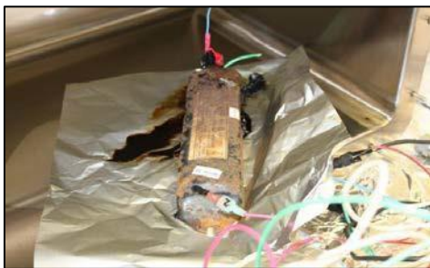
Above: Picture of ruptured fluorescent light
