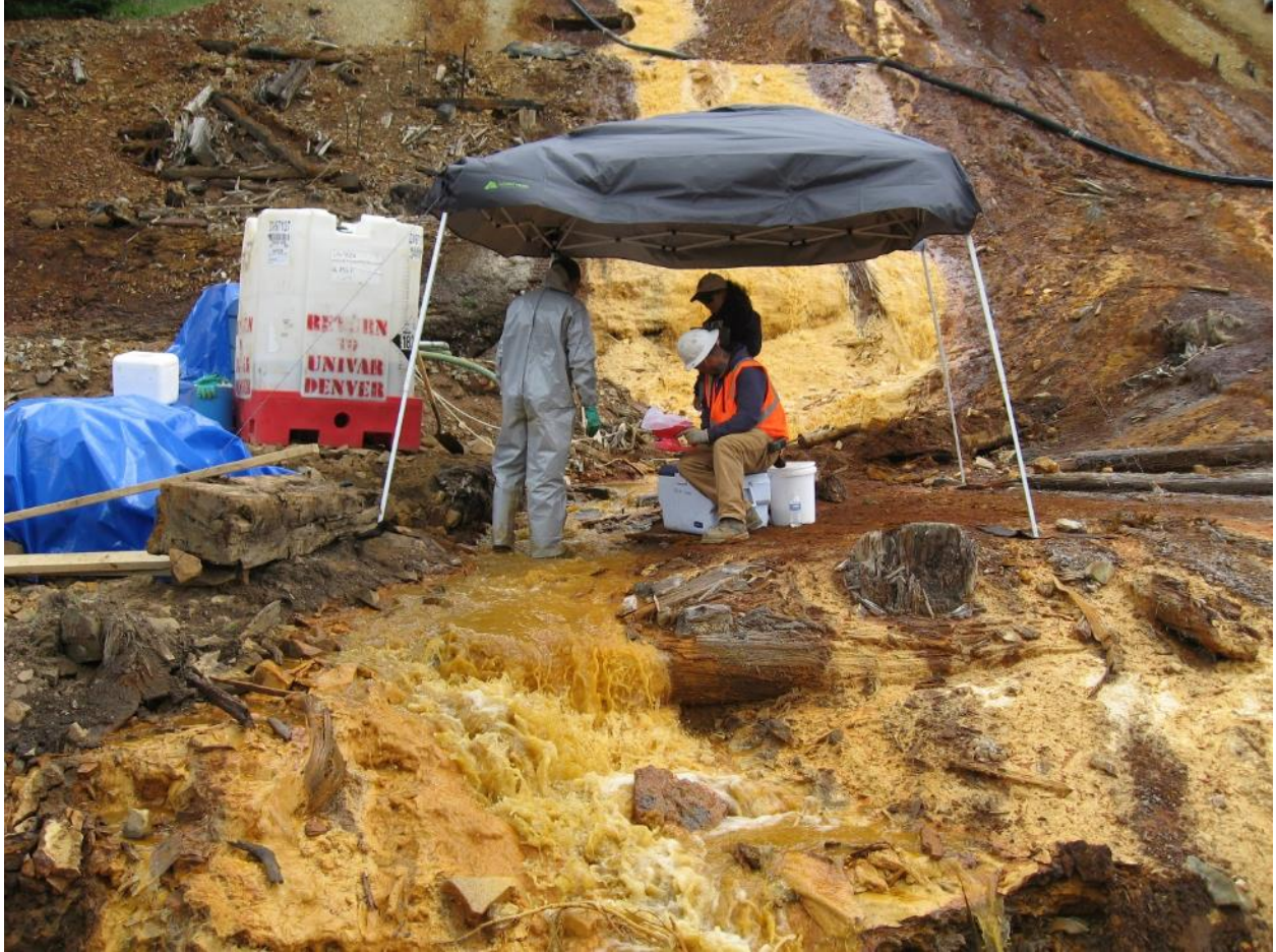
Sodium hydroxide addition upstream and flocculent addition below – pH raised from @ 3 su to 7 su
