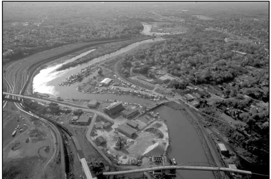
The 2005-2007 Legacy Act cleanup of the Ashtabula River removed 500,000 cubic yards of sediment contaminated with 25,000 pounds of PCBs and other contaminants.
