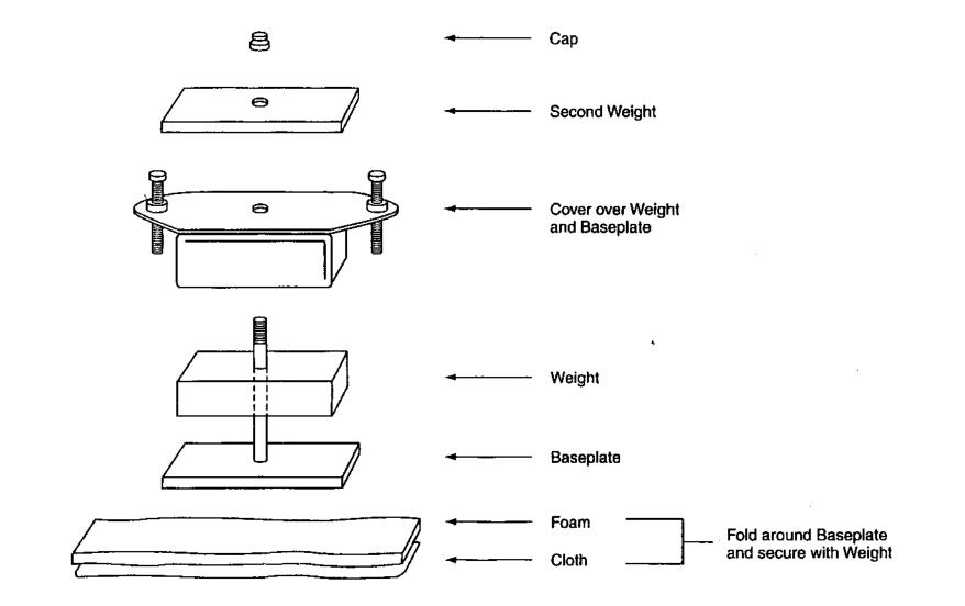
**Abrasion Tester with Abrasion Boat**
