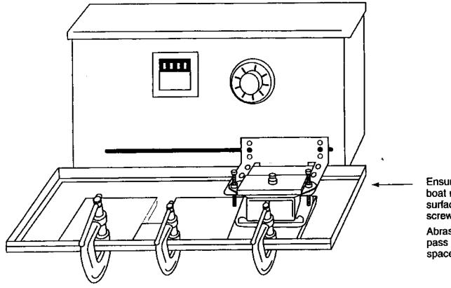
Ensure that abrasion boat rests lightly on surface by adjusting screw, if necessary.
