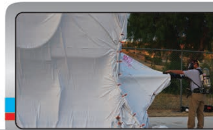
20 After the test is completed, and the methyl bromide has been sent through the activated carbon scrubber, personnel check the perimeter to ensure no methyl bromide is detected;
