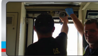
22 SO and railcar personnel open locked panels, check for methyl bromide before coupons and HOBOS can be recovered;
