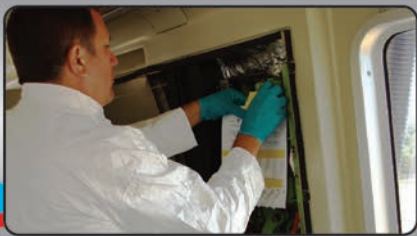
5 Placing coupons and HOBO (Temperature and Relative Humidity data logger) behind sealed electronics panels;
