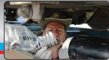
10 Placing time-series coupons in perforated pipe before fumigation begins;
