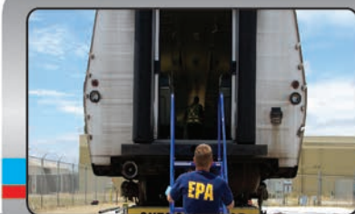
13 Last check of rail car with coupons and HOBOS, Mylar displacement bladders, humidifiers and heaters in place before wrapping the rail car;
