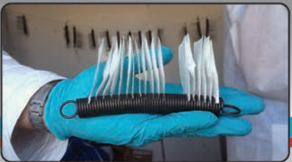
9 Time-series coupons placed on a spring (for stability) to be removed in 2-hour or 6-hour intervals;
