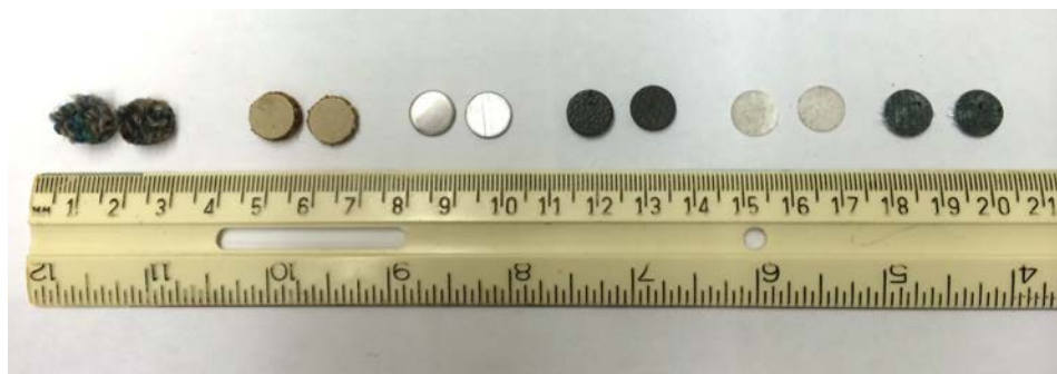
Rail car material coupons with surrogate spores from left to right: carpet, fiberglass, aluminum, rubber, Mylar, and plastic.
