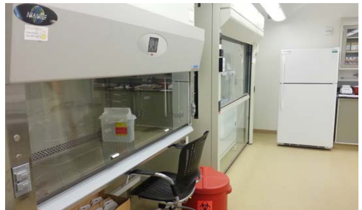
Certified Biosafety Cabinet and Chemical Fume Hood that houses a Janus Automated Workstation for high throughput sample processing.
