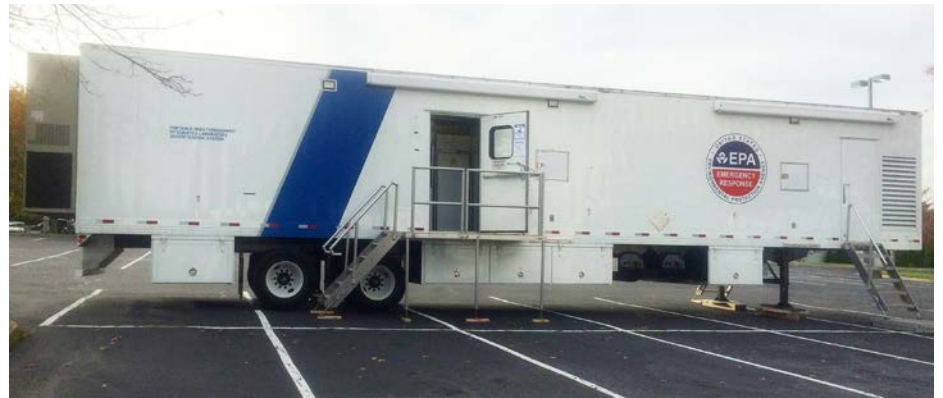
PHILIS Portable Analytical Laboratory (PAL) with 6 GC/MS on board.
