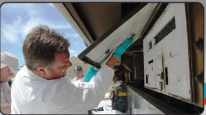
5 Placing coupons and HOBO (Temperature and Relative Humidity data logger) behind sealed electronics panels;
