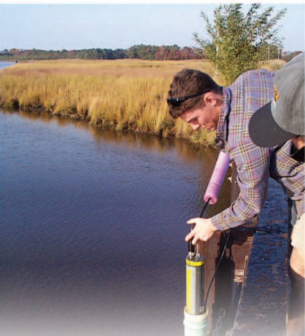
Deployment of continuous monitor (left). Specialized sensors are installed on an outboard boat to collect intensive water quality data over a large area in a short time (below).
