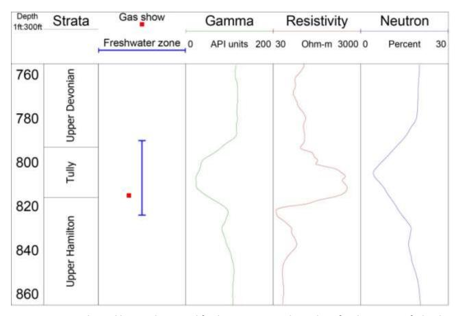
Figure 2. Geophysical logs and reported freshwater zone and gas show for the 760-860 ft depth interval in gas well 19484, Cortland County, New York
