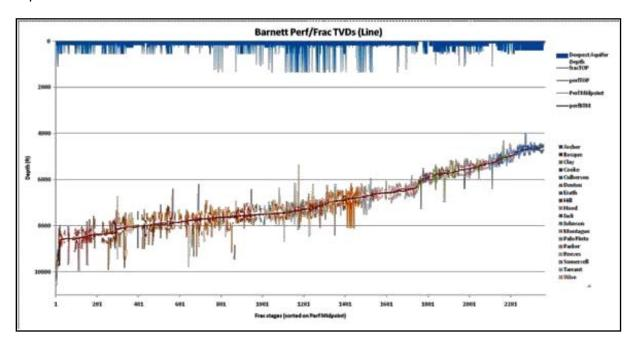
Figure 17. A compendium of microseismic fracture diagnostic results in the Barnett shale relative to known aquifers.
