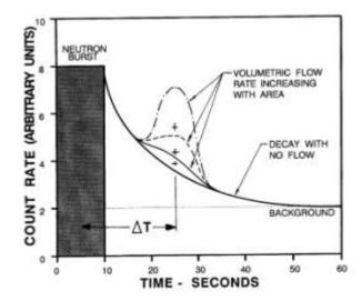
Figure 24. WFL Measurement Technique
