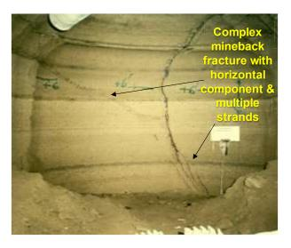
Figure 12. Mineback photograph of complex fracture
