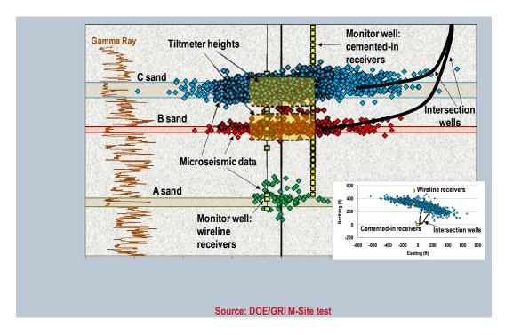
Figure 15. Overview of DOE/GRI M-Site hydraulic fracture diagnostics field test site.
