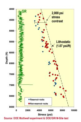
Figure 14. Measured stress profile in Mesaverde.
