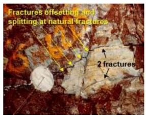
Figure 13. Mineback photograph of offsets & splitting.
