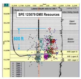
Figure 16. Example Haynesville shale microseismic data.
