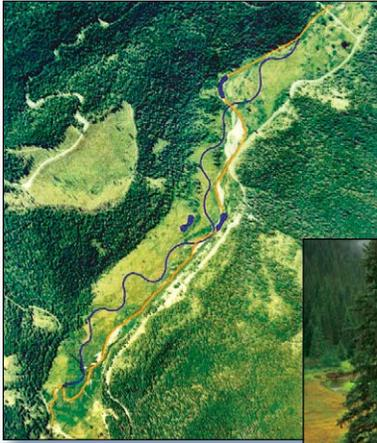
Figure 2. The Tepee Creek Meadows Restoration Project included reconstruction of stream meanders (blue) where the stream had been channelized (orange).
