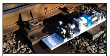
This small motor produces electricity from passing trains and could potentially power lights or signs.
