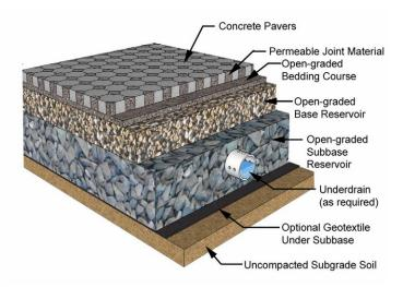
Above: System Components of Permeable Interlocking Concrete Pavement (PICP). The base layers of a permeable pavement system are similar for permeable pavers, porous asphalt, and pervious concrete. Each system has some variations which are important for structural integrity. Below: Pervious pavement in Portland, OR.
