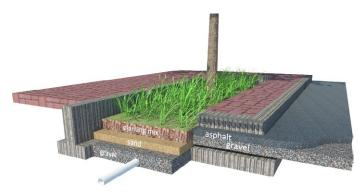
Treated stormwater is then either infiltrated into the ground as groundwater (infiltration planters) or discharged into a conventional storm sewer pipe (flow-through planters), where infiltration is not appropriate.
