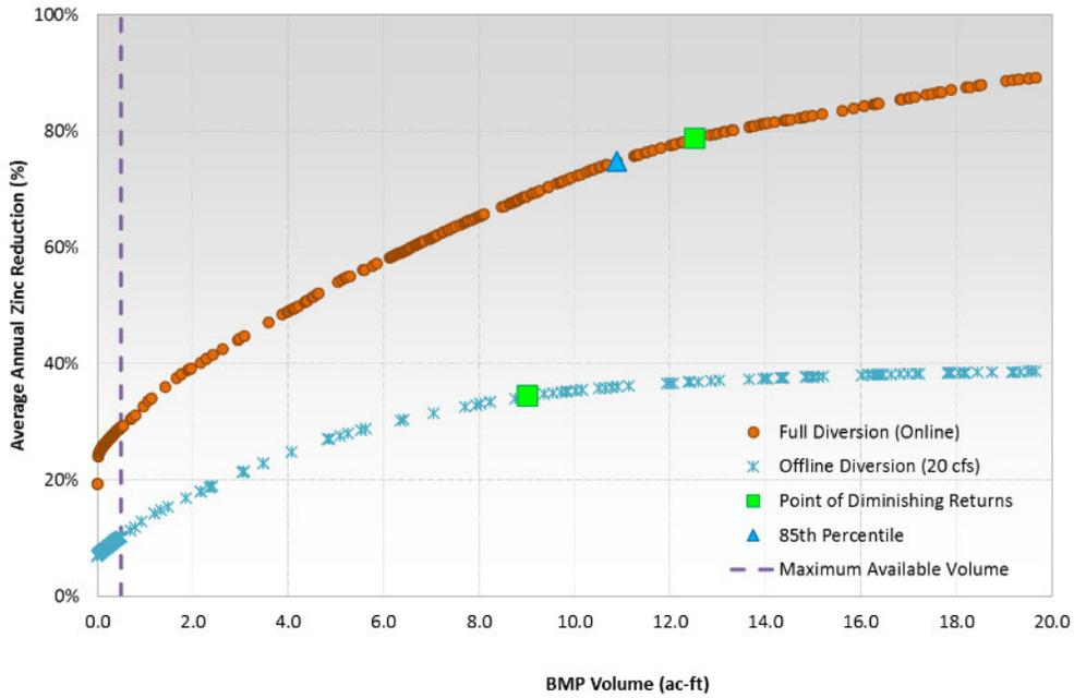
Figure 4-6. Infiltration gallery sizing optimization curve for Ozone Park (Scenario 1).
