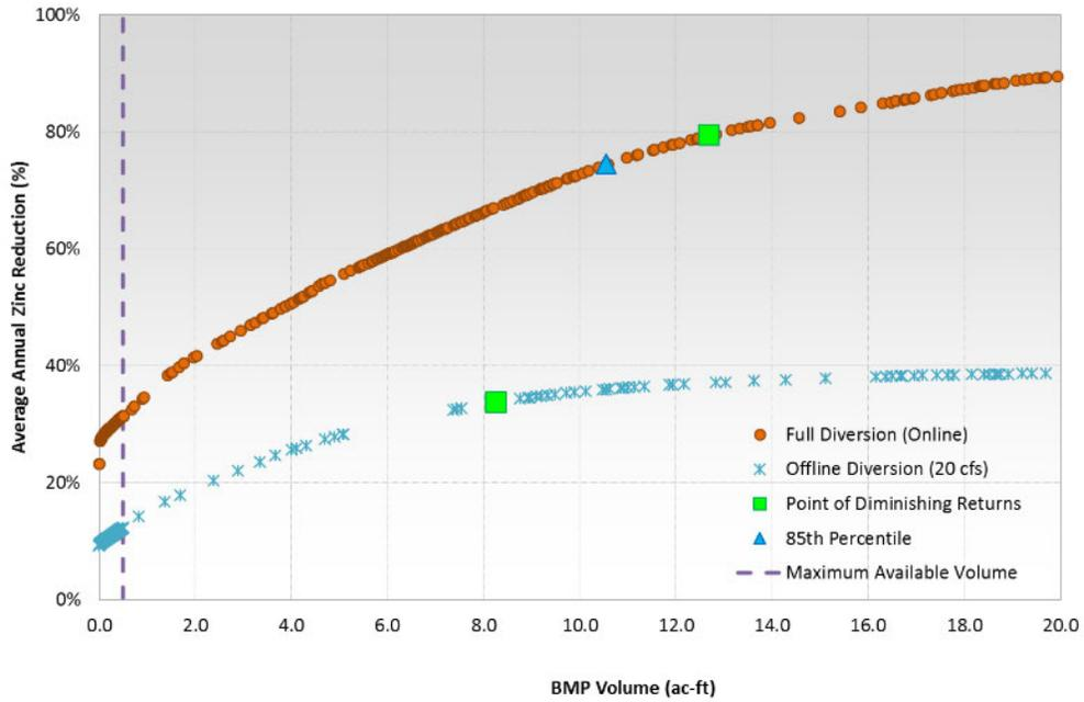
Figure 4-8. Infiltration gallery sizing optimization curve for Ozone Park (Scenario 3).
