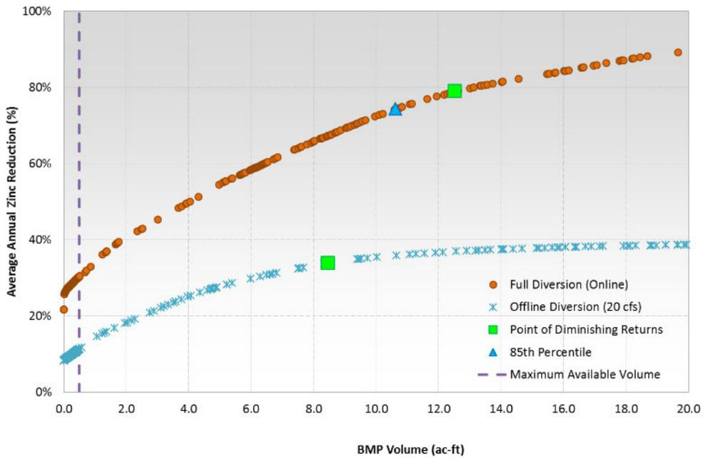
Figure 4-7. Infiltration gallery sizing optimization curve for Ozone Park (Scenario 2).
