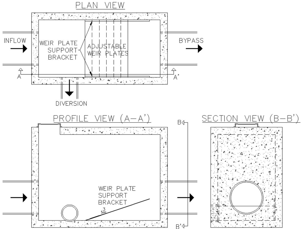
Figure 4-4. Typical diversion structure.
