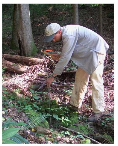
Figure 3-51 Using sounding rod and hand sledge hammer to estimate depth to bedrock and the groundwater table.
