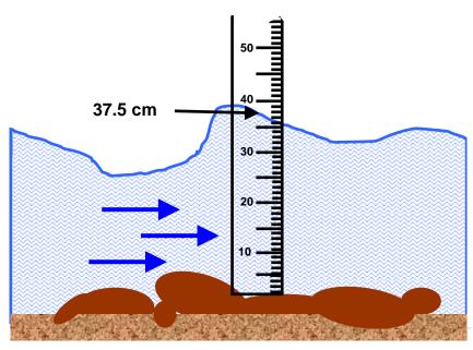
Figure 3-29 Schematic showing appropriate reading of water depth where water surface is turbulent.
