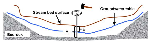
Figure 3-52 Cross-section of a dry channel illustrating depth to underlying bedrock (A) and depth to the groundwater table (B).
