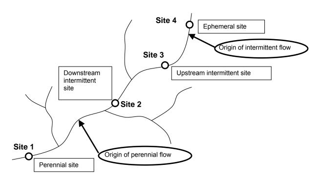
Figure 2-6 Schematic of headwater channels showing numerical designation and position of study sites relative to origins of intermittent and perennial flow.
