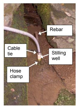
Figure 3-7 Water sensor securely attached to rebar above and below stilling well.
