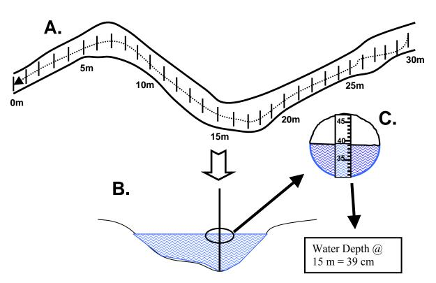
Figure 3-27 Overhead view of study reach showing locations for water depth measurement (vertical black tick marks) along the reach thalweg (dotted line). Water is flowing from right to left. (A.) overhead view of study reach (B.) channel cross-section, and (C.) lateral close-up of depth.
