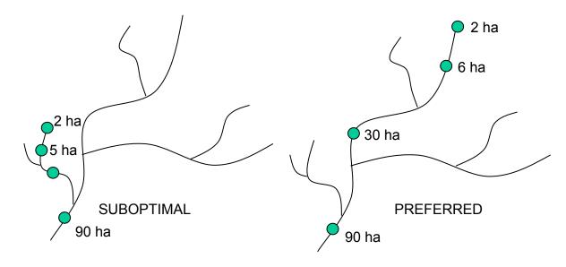
Figure 2-4 Schematic showing suboptimal and preferred longitudinal positioning of sites along headwater channels to maximize the range of hydrologic permanence across study sites. Hypothetical drainage areas are shown to further illustrate spatial hierarchy.
