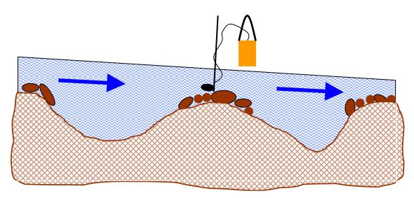
Figure 3-41 Longitudinal section across the channel thalweg showing orientation of the velocity probe for measurements.
