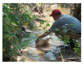
Figure 4-15 Carefully adding water to the wash basin before sample elutriation.
