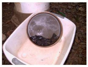
Figure 4-19 Sieve contents condensed for transfer to sample bag.
