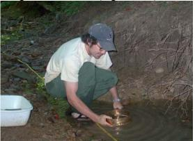
Figure 4-18 Washing sieve contents to one side by gentle agitation while sieve is partially submerged.
