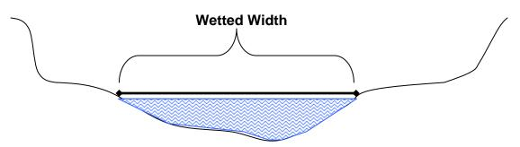
Figure 3-31 Channel cross-section illustrating wetted width.
