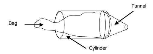
Figure 3-43 Bag meter used to measure water velocity.
