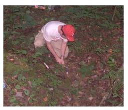
Figure 3-55 Tapping core vertically into streambed.
