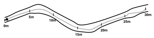
Figure 3-40 Plan view of study reach showing measurement locations (vertical black tick marks) for current velocity measurements. Flow is from right to left and the dotted line represents the thalweg.
