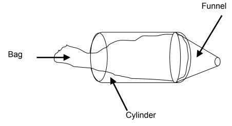
Figure 3-48 Bag meter used to measure discharge.
