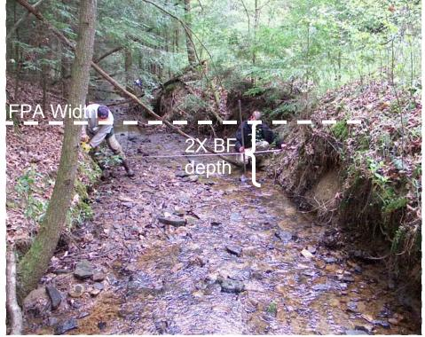
Figure 3-39 Photograph illustrating flood-prone area (FPA) width.
