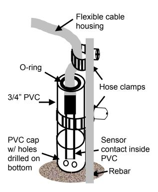
Figure 3-6 Schematic showing assembly of stilling well and contact end of water sensor.
