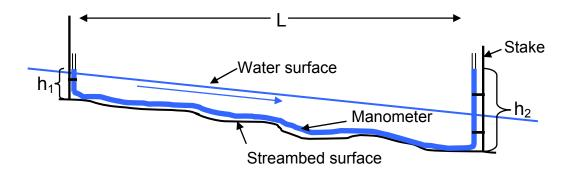
Figure 3-26 Longitudinal section of channel showing position of manometer and points of measurement to calculate slope (redrawn fro Gordan et al. 1992). Blue arrow shows direction of flow. L = horizontal length,  $h_1$  = height at the upstream end and  $h_2$  = height at downstream end.
