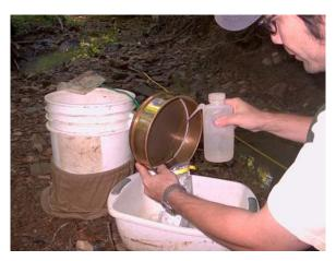
Figure 4-20 Sieve contents rinsed into sample bag (over basin) using ethanol squirt bottle.
