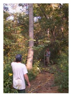
Figure 3-23 Crew members measuring slope of intermittent stream.
