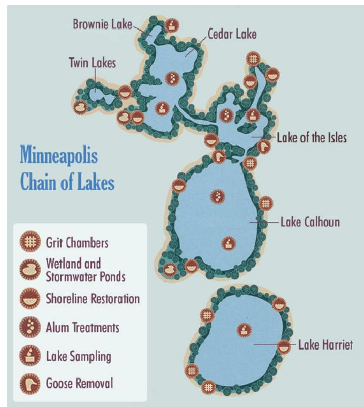
through the watershed. Projects included a two-cell wet pond at Cedar Lake and a three-cell sediment basin adjacent to Lake Calhoun. Other efforts focused on extensive shoreline erosion prevention measures from Cedar through Harriet Lakes, followed by the installation of numerous grit chambers, pocket wetlands, and improved street-sweeping practices. Alum treatments (using a nontoxic material to control internal
