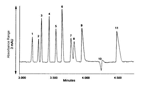
Electrolyte: 4.7 mM Na<sub>2</sub>CrO<sub>4</sub>/4.0 mM TTAOH / 10 mM CHES / 0.1 mM Calcium Gluconate
