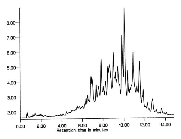
Toxaphene analyzed on an SPB-608 fused-silica open-tubular column. The GC operating conditions were as follows: 30-m x 0.53-mm ID SPB-608. Temperature program: 200  $^{\circ}$ C (2 min hold) to 290  $^{\circ}$ C at 6  $^{\circ}$ C/min.
