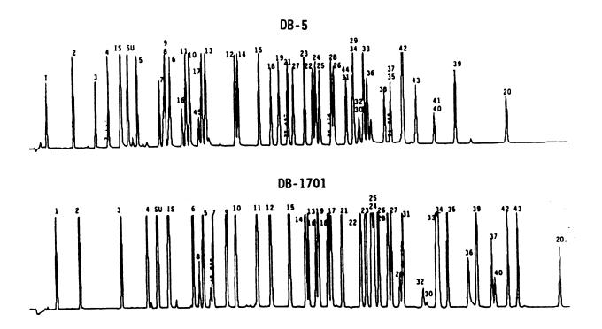
Organochlorine pesticides analyzed on a DB-5/DB-1701 fused-silica open-tubular column pair. The GC operating conditions were as follows: 30-m x 0.53-mm ID DB-5 (0.83- $\mu$ m film thickness) and 30-m x 0.53-mm ID DB-1701 (1.0- $\mu$ m film thickness) connected to an 8-in. injection tee (Supelco Inc.). Temperature program: 140 °C (2 min hold) to 270 °C (1 min hold) at 2.8 °C/min.
