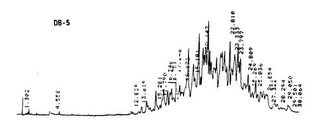
Strobane analyzed on a DB-5/DB-1701 fused-silica open-tubular column pair. The GC operating conditions were as follows: 30-m x 0.53-mm ID DB-5 (1.5- $\mu$ m film thickness) and 30-m x 0.53-mm ID DB-1701 (1.0- $\mu$ m film thickness) connected to a J&W Scientific press-fit Y-shaped inlet splitter. Temperature program: 150 °C (0.5 min hold) to 190 °C (2 min hold) at 12 °C/min then to 275 °C (10 min hold) at 4 °C/min.
