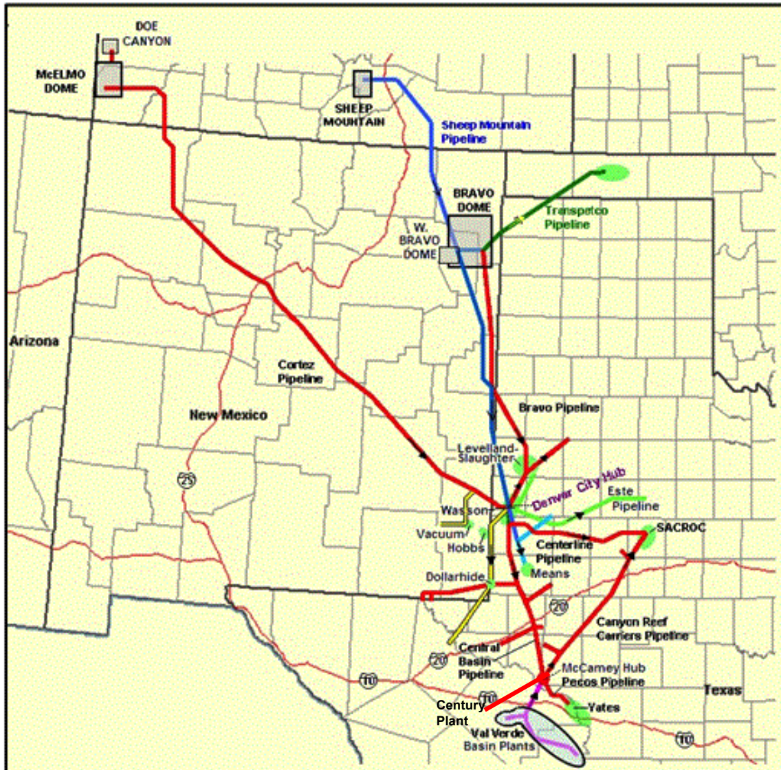
Figure A1-2 Permian Basin CO2 Pipeline Delivery System
