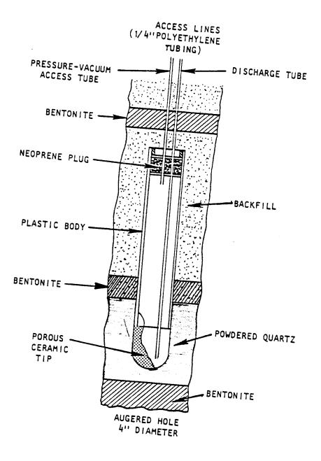
Figbre 9-6. Typical Ceramic Cup Pressure/Vacuum Lysimeter
