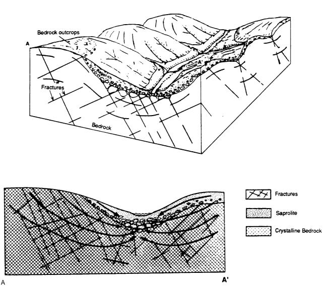
Note: In areas of fractured bedrock, flow through fractures is often greater than flow through the bedrock matrix. Flow through these fractures may not conform to Darcy's Law. The above flow lines represent generalized flow paths rather than quantitative flow lines used in a flow net.
