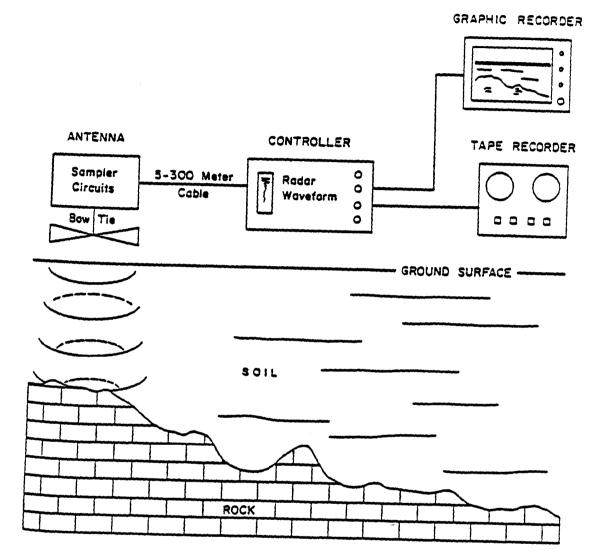
Figure C-4. Block diagram of ground penetrating radar system. Radar waves are relfected from soil/rock interface.
