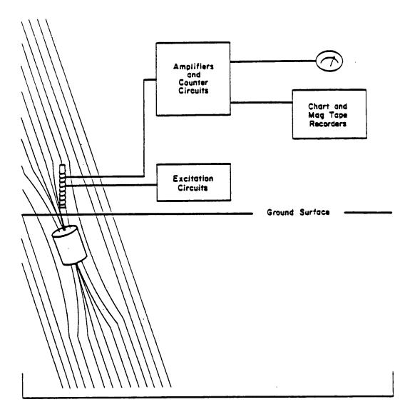
Figure C-5. Simplified block diagram of a magnetometer. A magnetometer senses change in the earth's magnetic field due to buried iron drum.
