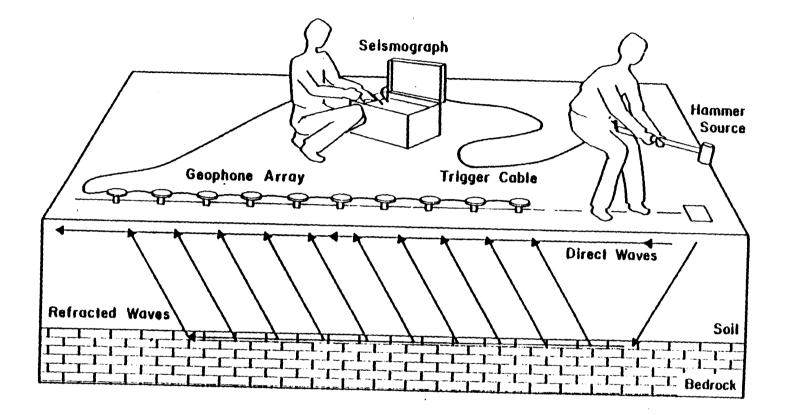
Figure C-2. Filed layout of a 12-channel seismograph showing the path of direct and refracted seismic waves in a two-layer soil/rock system.
