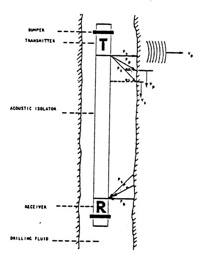
Figure C-12. Diagram of three-dimensional velocity tool (courtesy of Seismograph Service Corporation, Birdwell Division).
