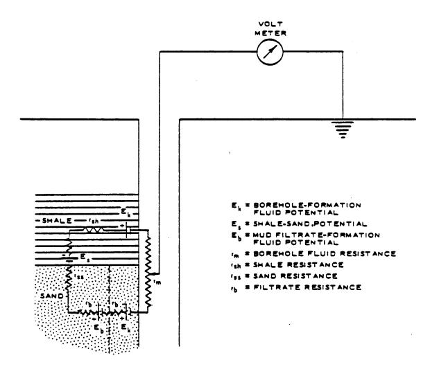
Figure C-6. Conceptual equivalent circuit for self-potential data (prepared by the Waterways Experiment Station, U.S. Army Corps of Engineers, Vicksburg, Mississippi).
