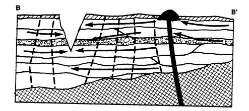
Schematic Diagram of Ground Water Flow Regime Through a Saturated Cross Section
