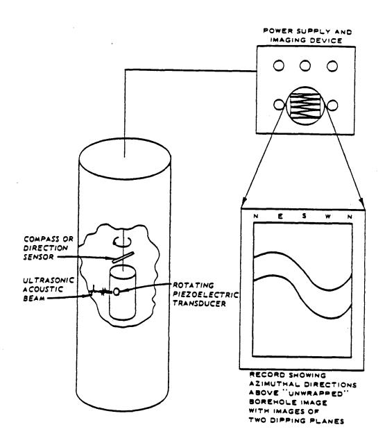
Figure C-II. Sonic imagery logger (prepared by the Waterways Experiment Station, U.S. Army Corp of Engineers, Vicksburg, Mississippi).
