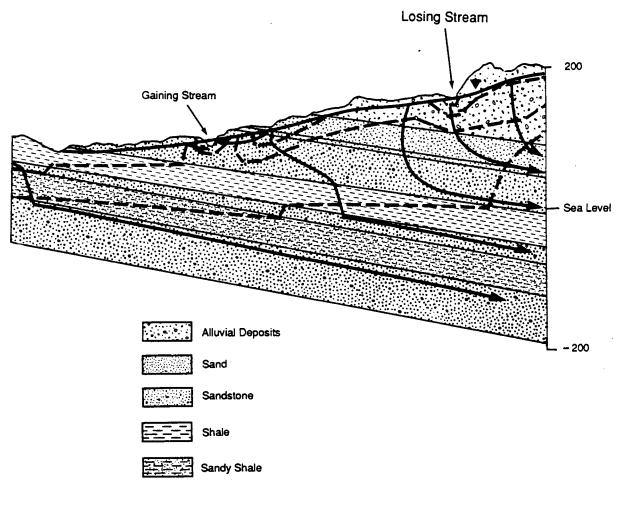
Note: Regional flow based on high recharge in hills which are not shown in this diagram.
