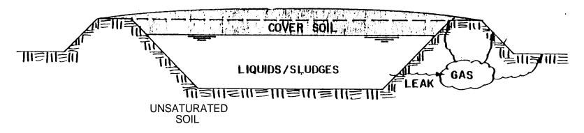
Figure 11-2. Subsurface Gas Generation/Migration from Tanks and Units Closed as Landfills (Note: Gas may also migrate slowly through cover soil.)
