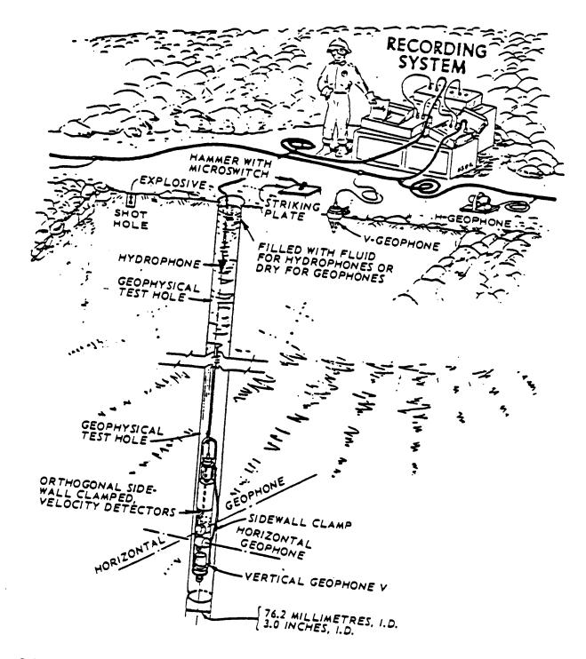
Figure C-9. Downhole survey techniques for P-wave data (prepared by the waterways Experiment Station, U.S. Army Corps of Engineers, Vicksburg, Mississippi).
