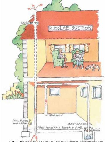
Note: This diagram is a composite view of several mitigation options. The typical mitigation system usually has only one pipe penetration through the basement floor; the pipe may also be installed on the outside ohe house.
