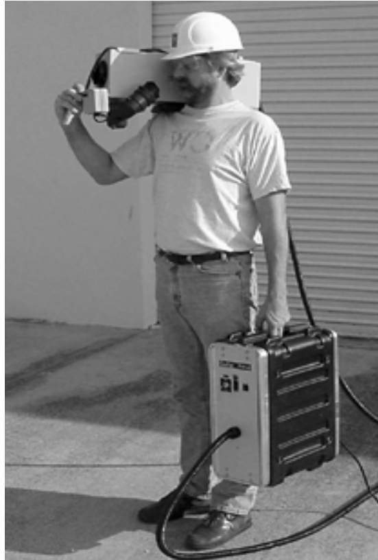
FIGURE 4. The New Air-Cooled GasVue TG-30 System
