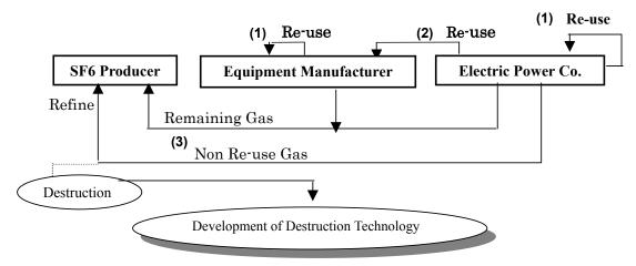
*Fig.6-1: SF*<sup>6</sup> *recycling flow*
