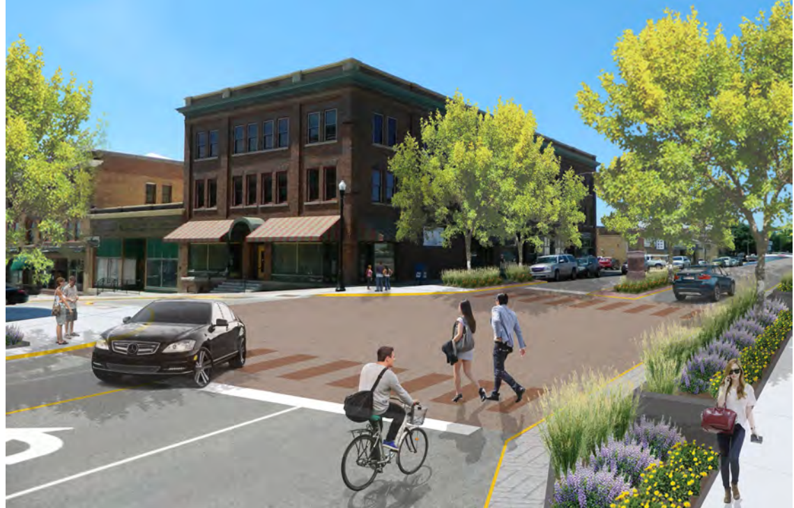
Figure 18: Design concept for the intersection of East Capitol Avenue and Upper Pierre Street. A colored and textured intersection makes pedestrian crossings more visible. Stormwater planters and street trees have been added along the rights-of-way and in a center median. These elements work together to calm traffic, making bicyclists and pedestrians crossing the street safer.
