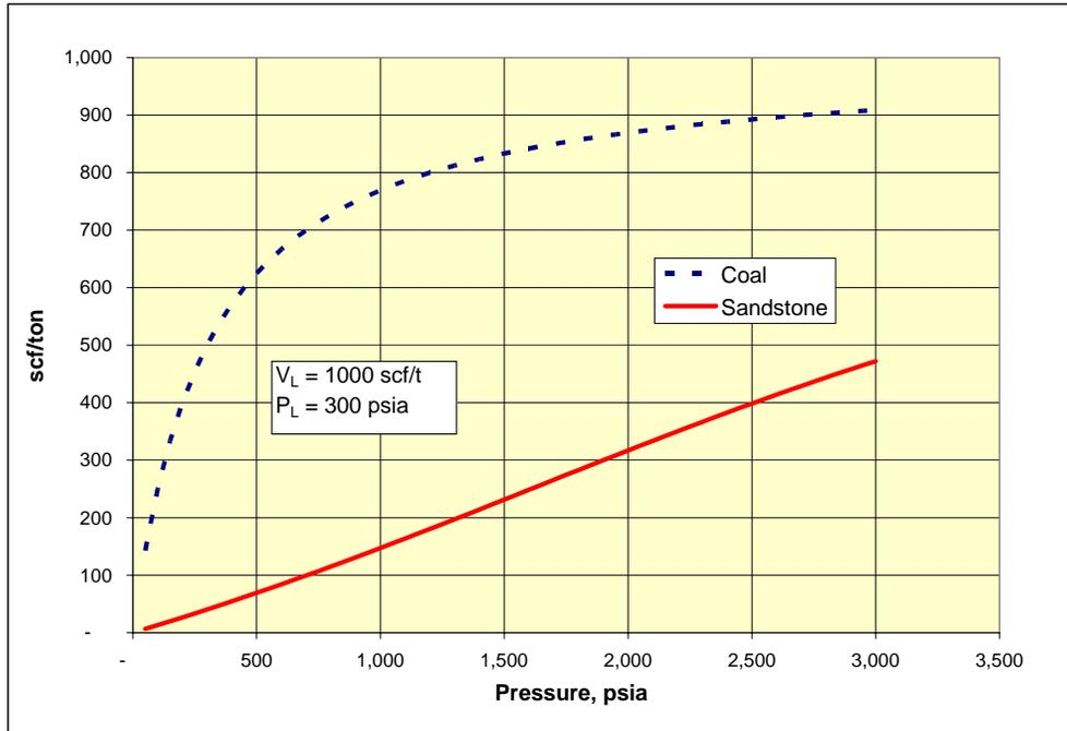
**Figure 4. Typical adsorption isotherms as a function of coal rank (GRI, 1996)<sup>10</sup>**
