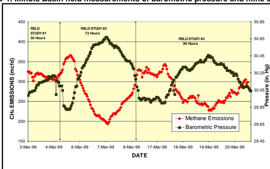
Correlating gas flow rates to barometric pressure is critical for obtaining representative field measurements for decline curve validation. The correlation between gas flow and barometric pressure is shown in **Figure D-2**. The linear regression equation describing the relationship resulted in a correlation coefficient ( $R^2$ ) equal to 0.92.
