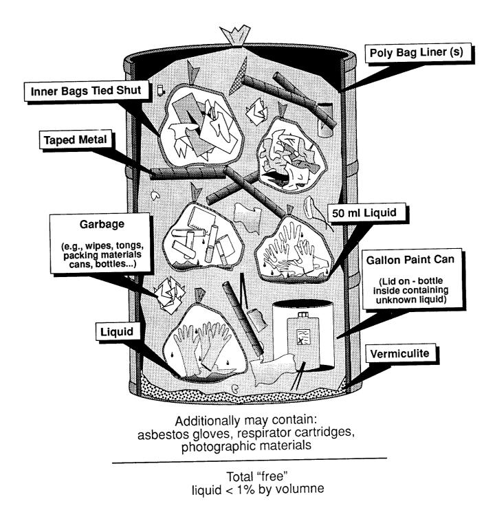
Figure 1-1. The worst-case drum of heterogeneous wastes.
