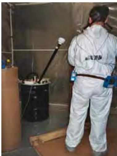
**Photograph 3. 5: Feeding Bulbs into the Manufacturer C Device**
