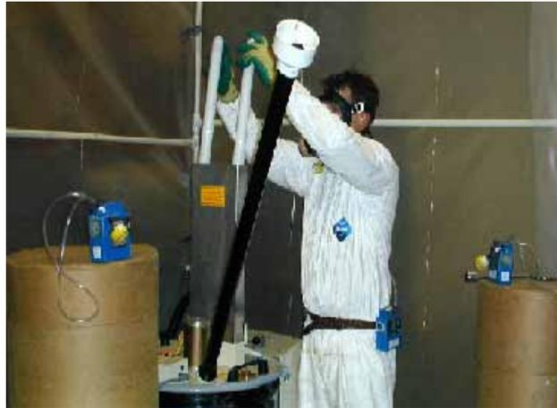
**Photograph 3. 6: Crushing of U-Tubes - Manufacturer C Device**
