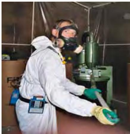
**Photograph 3. 3: Feeding Bulbs into the Manufacturer A Device**
