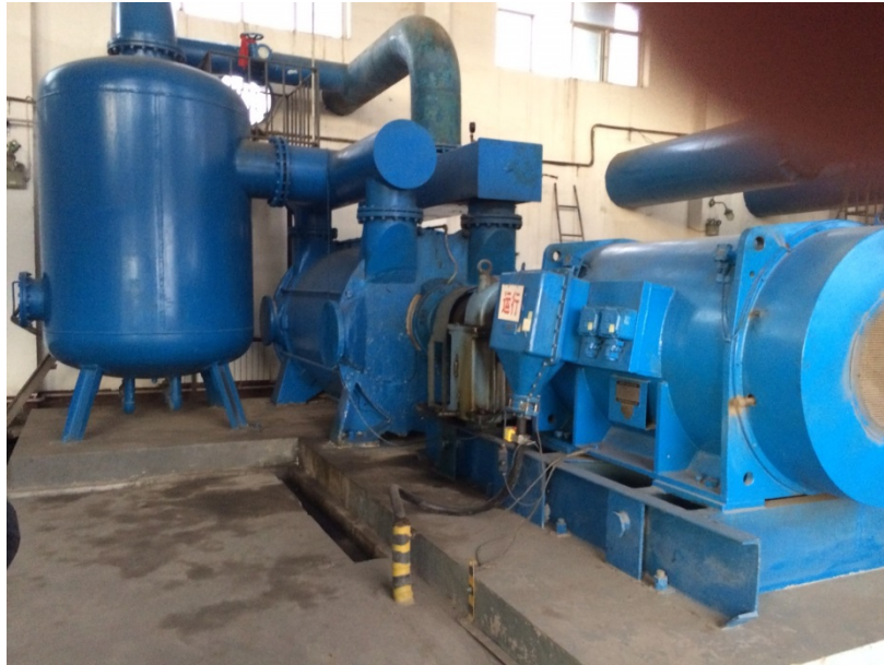
Figure 4-2: Vacuum pump at the Pingshang Mine
