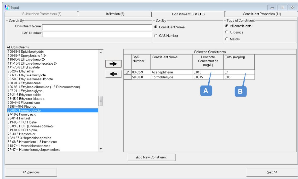
**Figure 3-22. Input: Constituent List (10): Enter Leachate Concentrations for WMUs and Structural Fills.**
