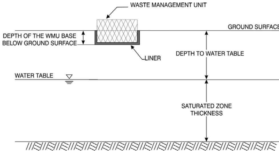
Figure 4-2. WMU with base below ground surface.
