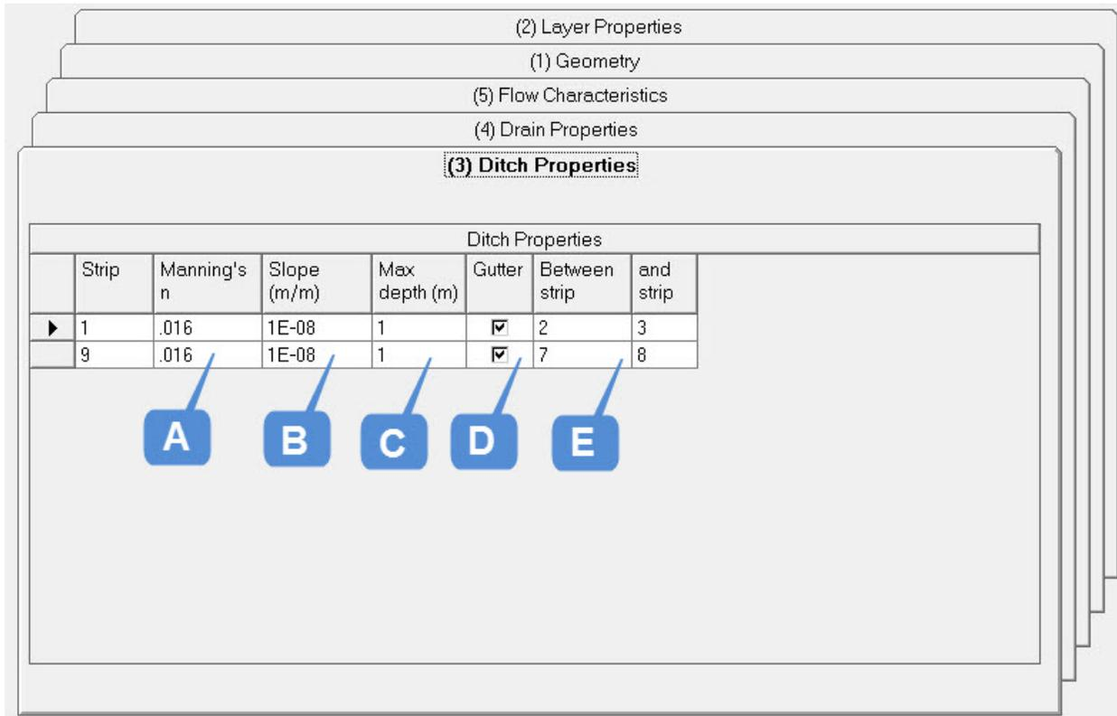
**Figure 3-13. Input: Source Parameters (7) for Roadways: Ditch properties.**
