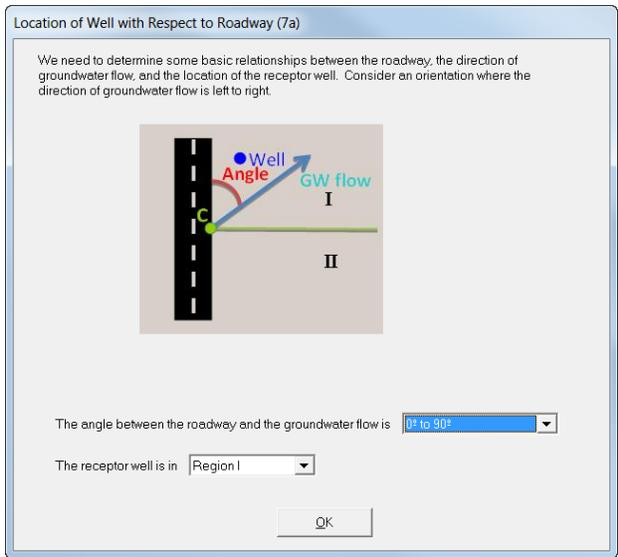
Figure C-39. Location of Well with Respect to Roadway (7a).
