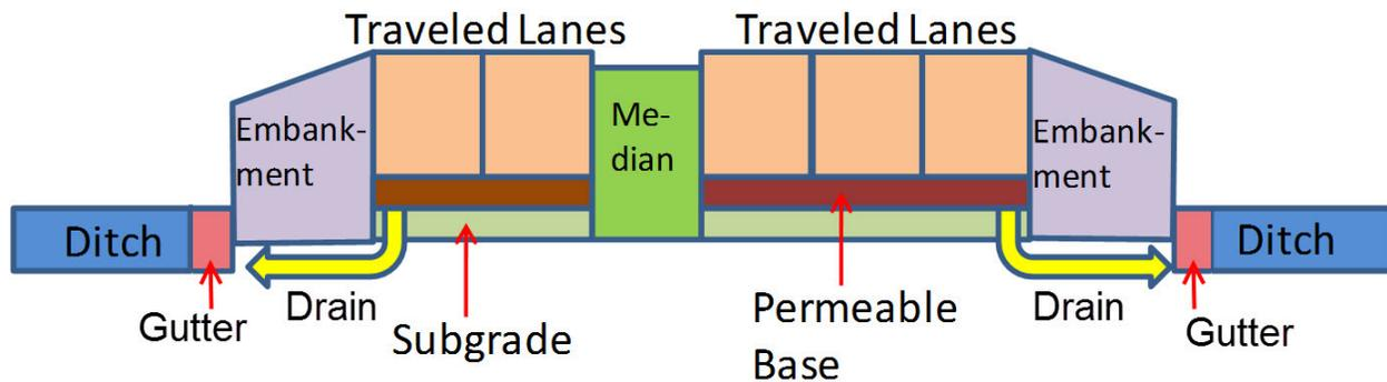
**Figure 2-3. A typical cross section of a roadway.**
