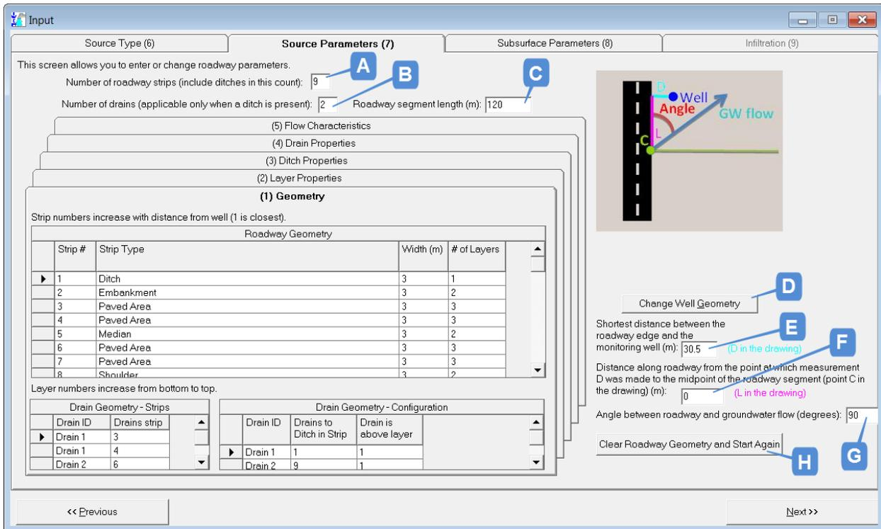
**Figure 3-10. Input: Source Parameters (7) for Roadways: Overview.**
