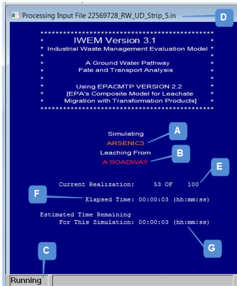
**Figure 3-33. Evaluation: EPACMTP dialog box displayed during model execution.**
