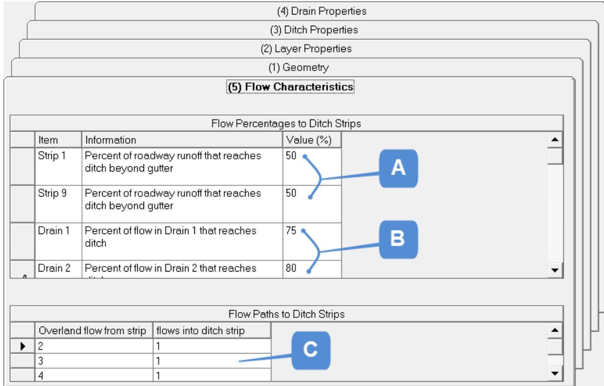
Figure 3-15. Input: Source Parameters (7) for Roadways: Flow Characteristics.
