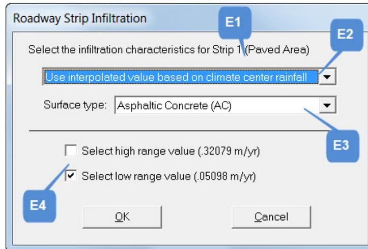
**Figure 3-20. Default roadway strip infiltration dialog.**
