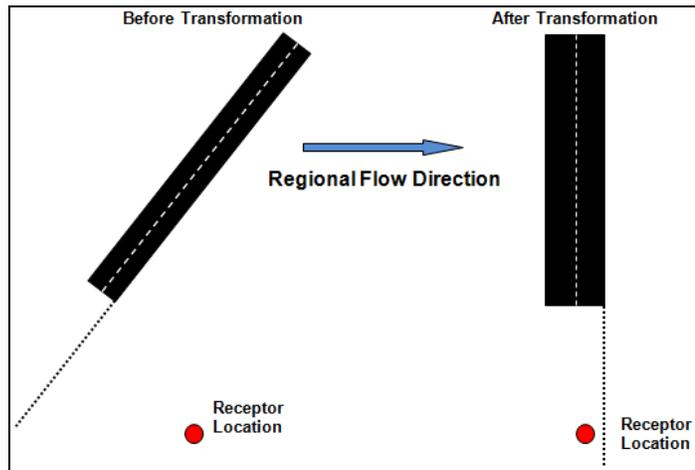
**Figure 4-8. Example of invalid receptor location after geometric transformation.**
