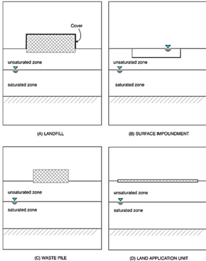
Figure 4-1. WMU types modeled in IWEM.
