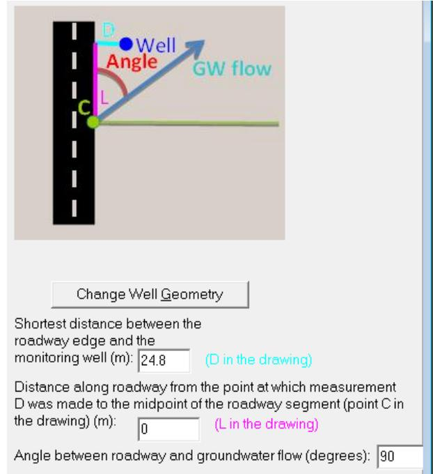
**Figure C-5. Source Parameters (7) – Well Geometry.**
