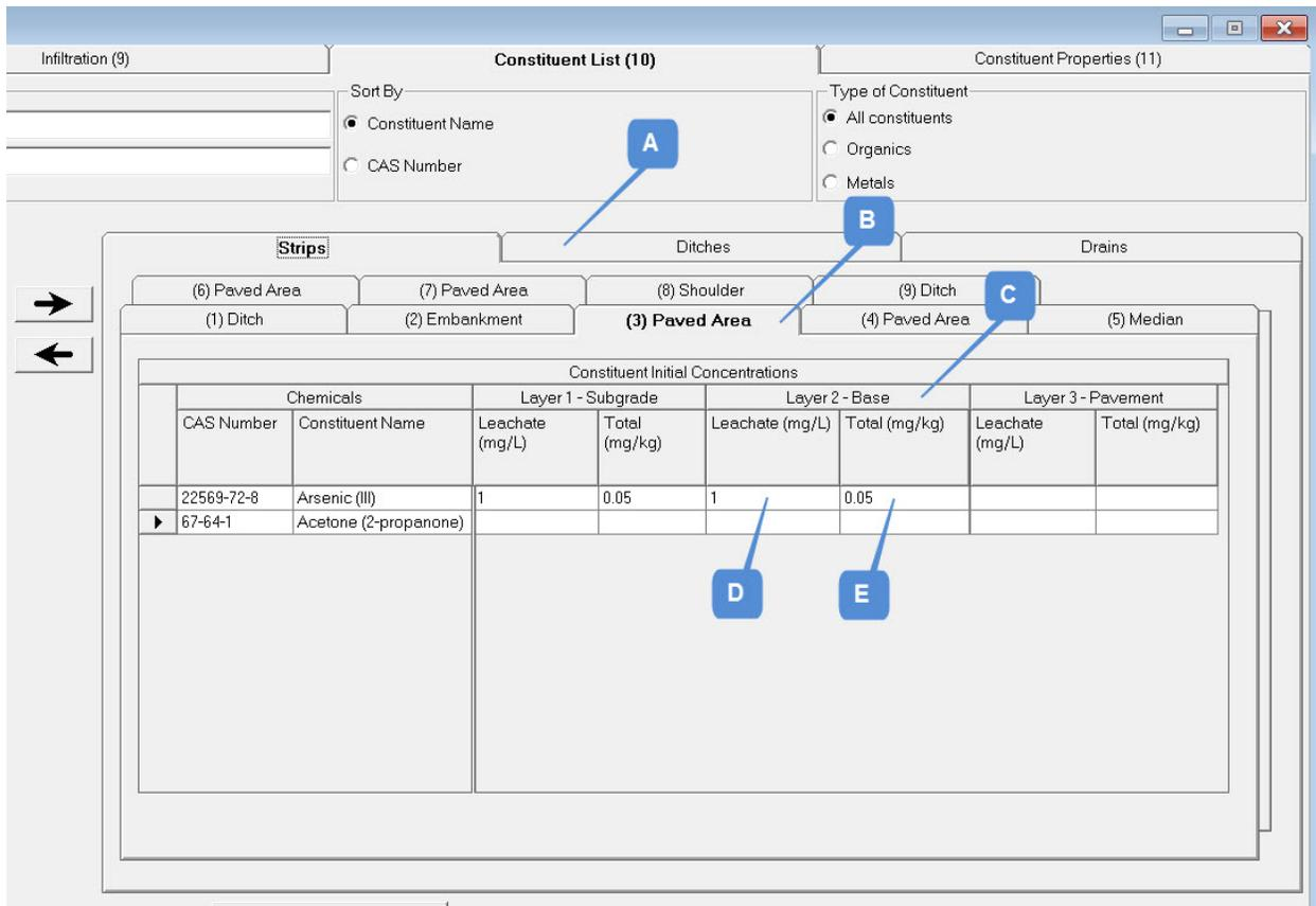
**Figure 3-23. Input: Constituent List (10): Enter Leachate Concentrations for Roadway Strips.**
