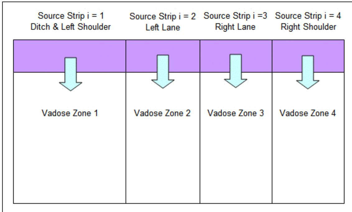
Figure 2-4. Modules of IWEM corresponding to multiple roadway-source strips.
