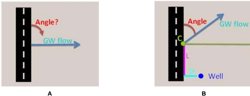
**Figure 4-6. Diagrams used by IWEM to specify roadway geometry.**
