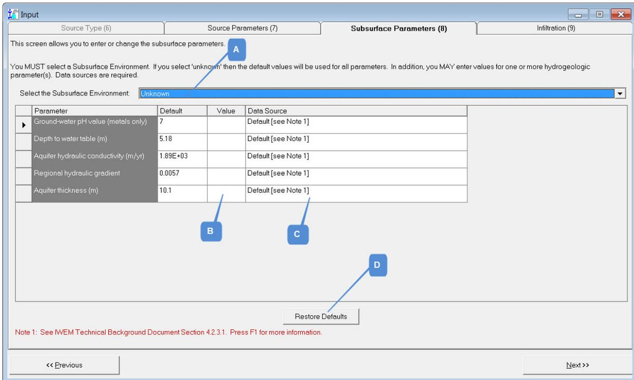
**Figure 3-16. Input: Subsurface Parameters (8).**
