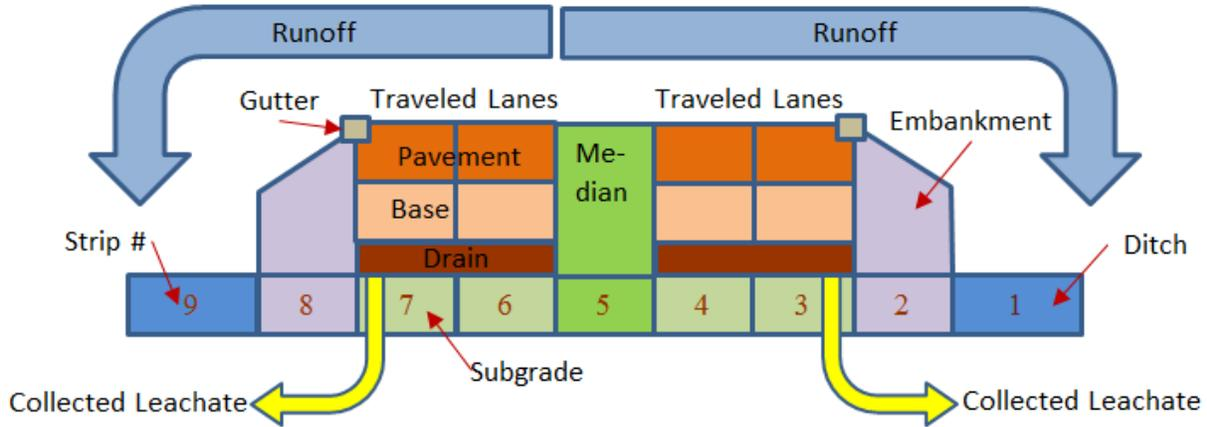
**Figure C-36. Cross Section of a Roadway Segment in Verification Case 4 with Two Symmetric Drainage Systems [not to scale]**
