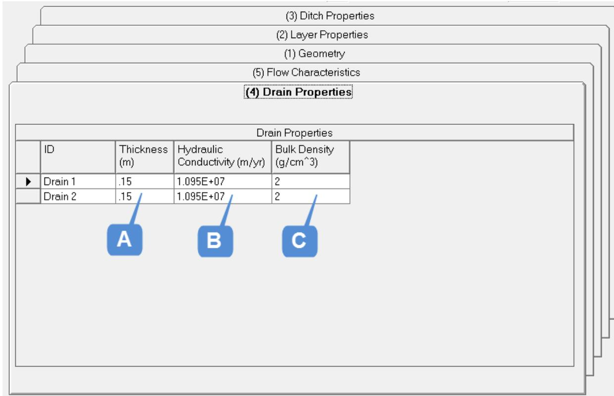
**Figure 3-14. Input: Source Parameters (7) for Roadways: Drain properties.**
