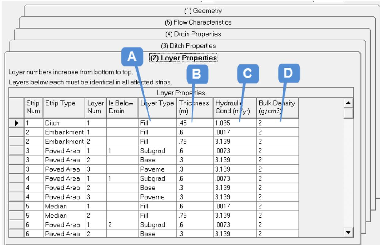
Figure 3-12. Input: Source Parameters (7) for Roadways: Layer properties.
