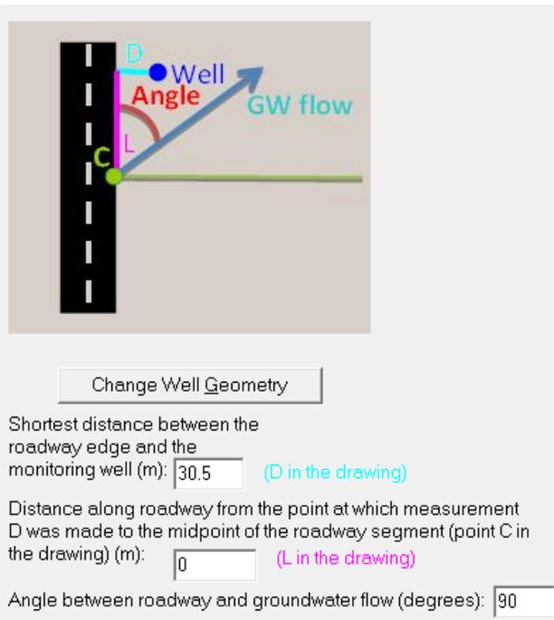
Figure C-40. Source Parameters (7) – Well Geometry.
