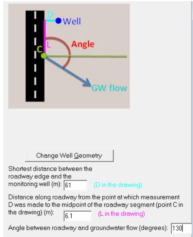
Figure C-15. Source Parameters (7) – Well Geometry.
