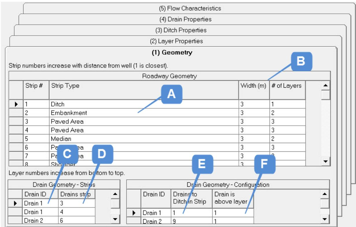
Figure 3-11. Input: Source Parameters (7) for Roadways: Geometry.
