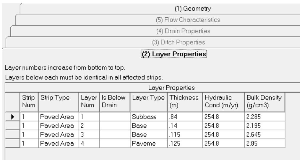
**Figure C-7. Source Parameters (7) – Layer Properties.**
