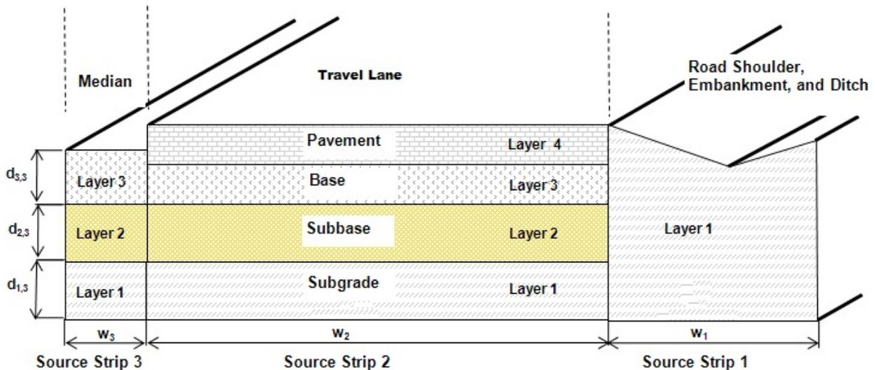
Figure 2-5. An example of layering in roadway-source strips.
