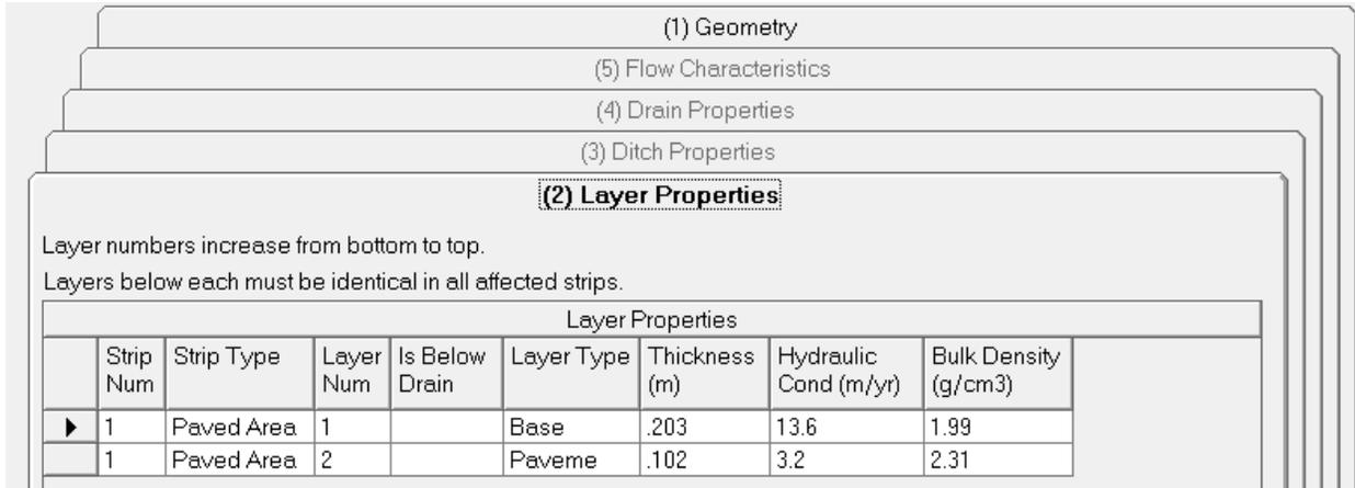
**Figure C-27. Source Parameters (7) – Layer Properties.**
