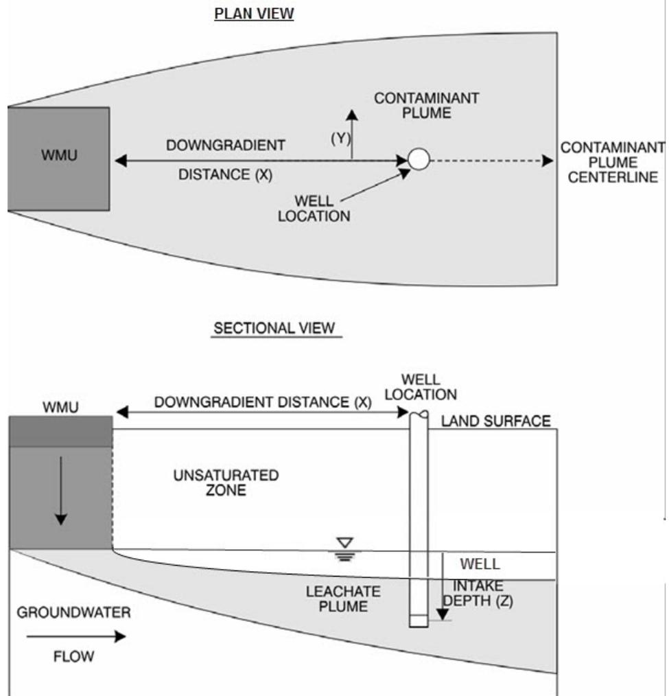
**Figure 4-3. Position of the modeled well relative to the WMU.**
