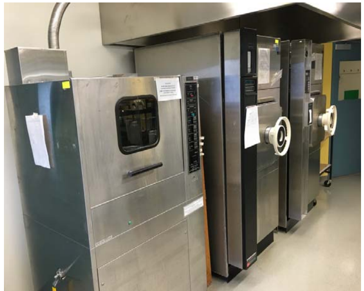
Figure 4: MEL's three autoclaves are manually controlled to ensure that water flow is not continuous.
