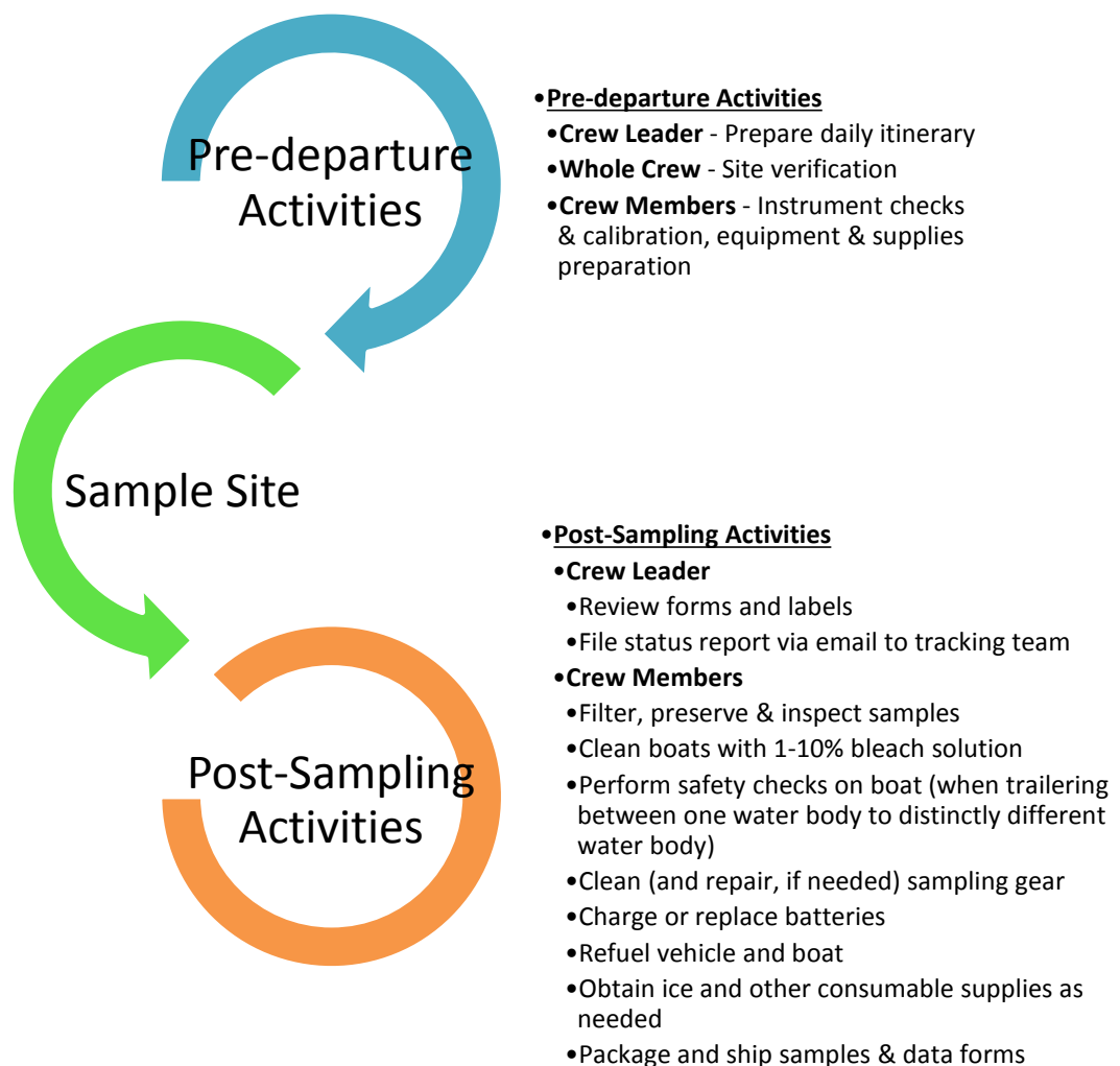
Figure 4.1 Overview of base site activities
