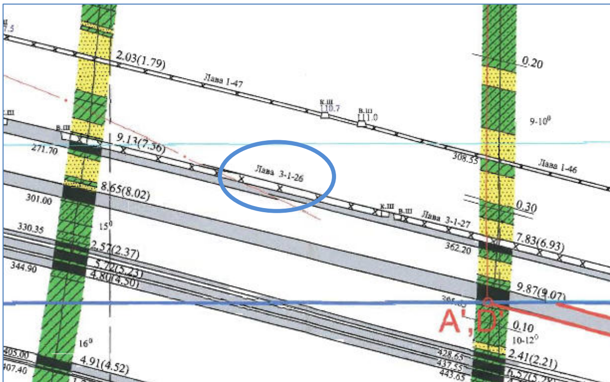
Figure 22. Panel 3-1-26; almost half of total coal thickness is left in the floor
