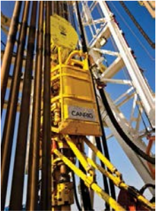
Electric driven Canrig Top Drive 4 times the torque power
