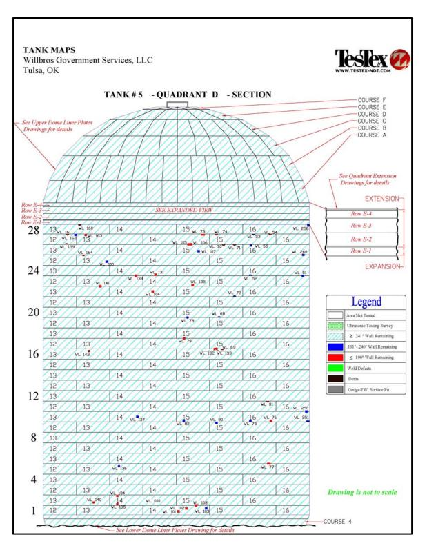
Figure 4-2. Example schematic drawing showing locations of flaws.
