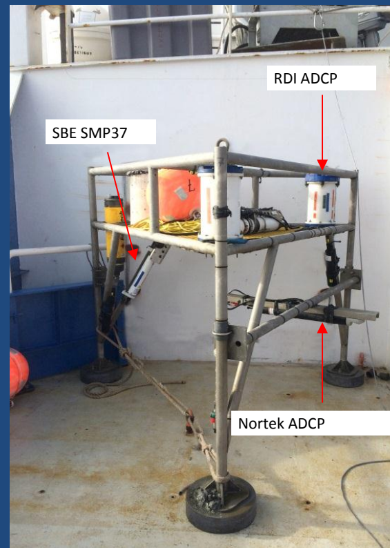
Left: Location of instruments in moored tripod frame Right: Close-up of the OBS3+ mounts
