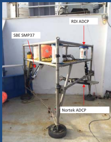
Left: Location of instruments in moored tripod frame Right: Close-up of the OBS3+ mounts
