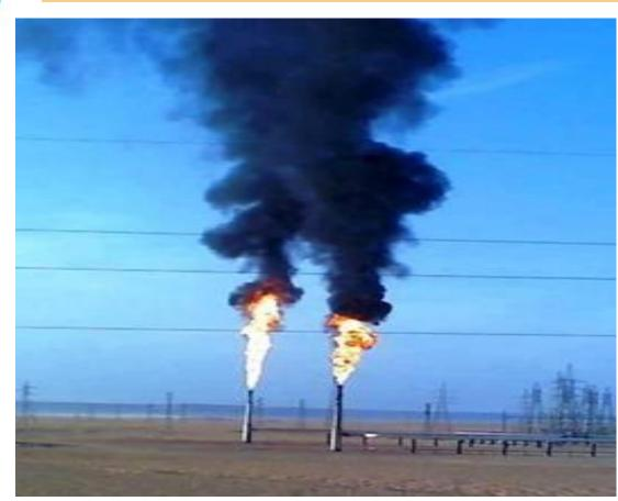
Picture of the flares at NC-115 location before the VRU's were installed
