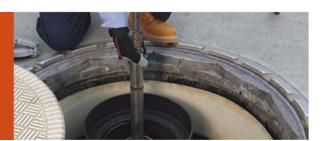
This method combines periodic tank tightness testing with monthly inventory control. Inventory control involves taking measurements of tank contents and recording amount received and pumped each operating day, as well as reconciling all this data at least once every 30 days. Every five years, this combined method must also include a tightness test, which is a sophisticated test performed by a trained professional.
