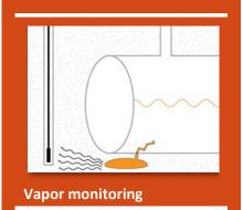
backfill or along pipe runs to intercept special chemicals that, in the event of a release, are detected in the sampling points.
