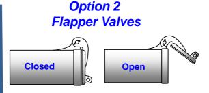
Flapper valves with a screen meeting local minimum size requirements can also be used to keep contamination out. Each valve design can get stuck open and therefore should be fitted with a screen inside. EPA recommends a #24 mesh screen. A flapper valve with no screen inside will trigger a significant deficiency.
