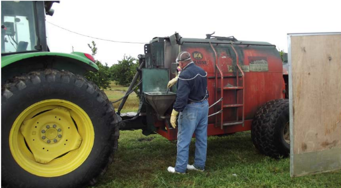
Figure 2: Mixing/Loading Wettable Powder in an On-board Inductor Tank
