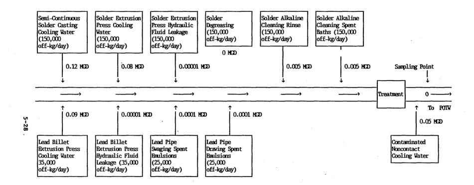
FIGURE 5-3. PROCESS FLOW DEAGRAM FOR A LEAD PIPE FORMING FACILITY
