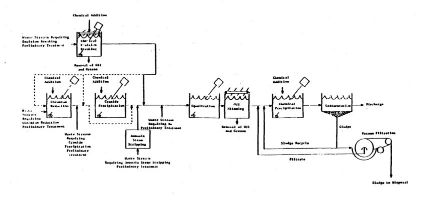
FIGURE 3-5. PSES/PSNS OPTION 1 AND 2 TREATMENT TRAIN FOR THE NONFERROUS METALS FORMING AND METAL POWDERS CATEGORY
