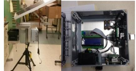
*Solar powered sensor device*
