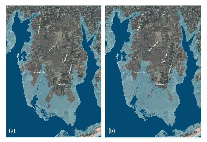
Figure 6. Areas of predicted inundation during a 100-year storm presently (a) and in 2050 after a sea level rise of 1.5 feet (b), consistent with the adjusted "Intermediate-High" NCA global sea level rise scenario).
