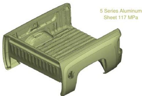
Figure 23. Material Map of Lightweighted Cargo Box
