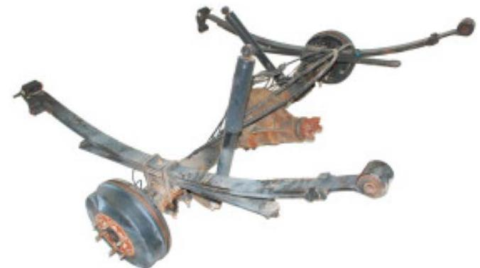
Figure 3. Rear Suspension Subsystem(Source: A2MAC1)
