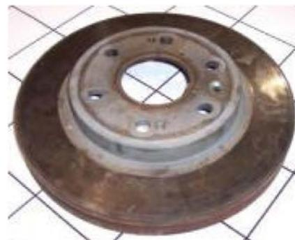
Figure 6. Front Rotor Current Component(Source: FEV North America, Inc.)
