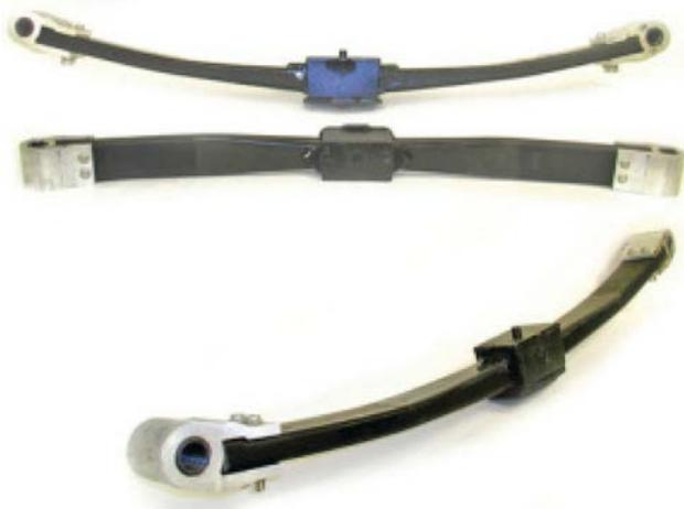
Figure 5. Rear Leaf Spring Mass Reduced Assembly(Source:<http://www.bing.com/images/search?q=Fiberglass+Leaf+Spring+Lightweight&FORM>)
