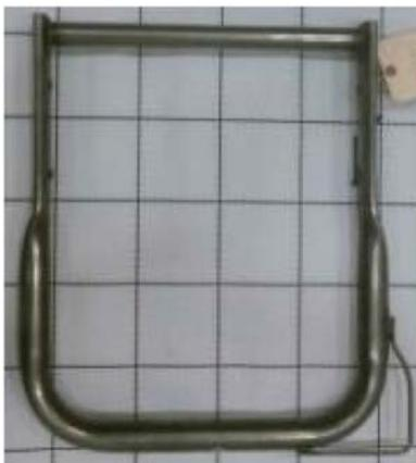
Figure 9. Rear 40% Seat Back Frame(Source: FEV North America, Inc.)
