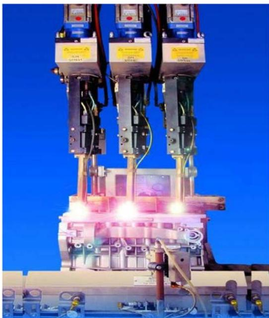
Figure 15. Plasma Transfer Wire Arc (PTWA)(Source:<http://www.geencarcongress.com/2009/05/ptwa-20090529.html>)
