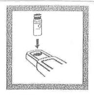
9. Within 3 minutes after the 3-minute reaction period, place the prepared sample in the cell holder.
