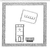
4. Fill another 1-cm/10-mL sample cell to the 10-mL line with sample (the blank). Cap.
