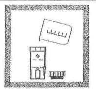
1. Fill a 1-cm/10-mL cell to the 10-mL line with sample.
