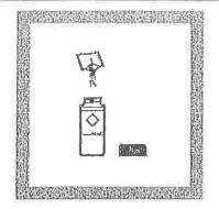
2. Add the contents of one DPD Total Chlorine Powder Pillow to the sample cell (the prepared sample). Cap and gently shake for 20 seconds.
