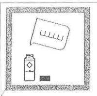
1. Fill a 10-mL cell to the 10-mL line with sample. Cap.
