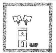
2. Add the contents of two DPD Total Chlorine Powder Pillows to the sample cell (the prepared sample). Cap the cell and shake gently for 20 seconds.
