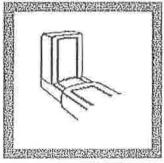
8. Tightly cover the cell with the instrument cap (flat side should face the back of the instrument).
