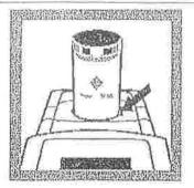
5. Place the blank into the cell holder, with the diamond mark facing you and the tab to the side.
