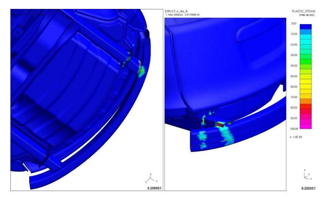
Figure 4.5.4.6.d shows the plastic strain for the impact beam for an offset impact.
