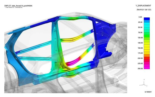
*Figure 4.3.8.f: Intrusion levels after 75°, side, pole impact on struck side – 5th percentile female*
