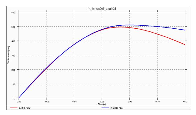
Figure 4.3.3.e: Vehicle displacement during  $30^\circ$ , left-side frontal impact – max dynamic crush = 500 mm
