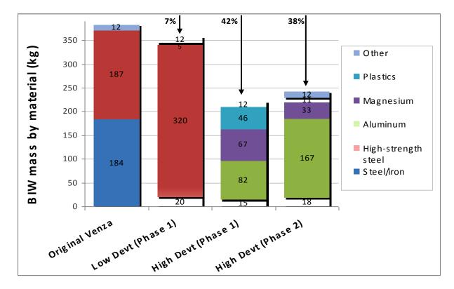
Figure 4.5.5.a: Venza, Phase 1, and Phase 2 vehicle body structure by material
