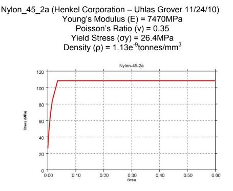
Figure 4.2.2.4.a: 45-2a nylon stress-strain curve
