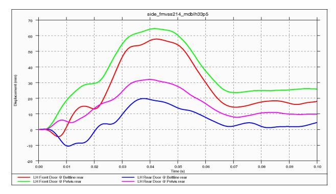
Figure 4.5.4.1.g: Relative Intrusion Displacements (Front/Rear Door)
