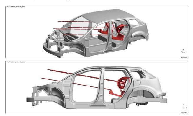
Figure 4.2.5.5.b: Rear seatbelt anchorage test model setup
