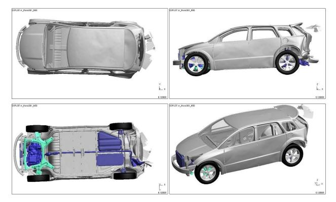
Figure 4.5.4.5.c: Vehicle Deformation (Barrier Blanked)
