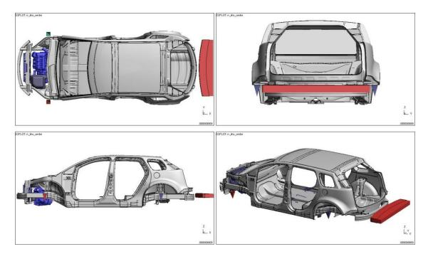
Figure 4.2.5.13.a: IIHS, low-speed rear test model setup ('full impact')
