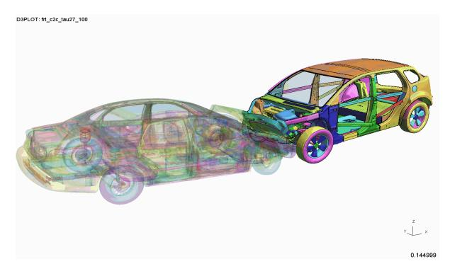
*Figure 4.4.9.e: Phase 2 HD vehicle to Ford Taurus crash simulation result – three-quarter view, opaque Taurus*
