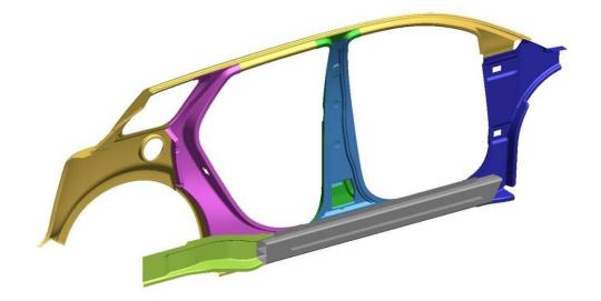
Figure 4.3.7.h: Main energy absorbing body structure parts for crabbed barrier impact
