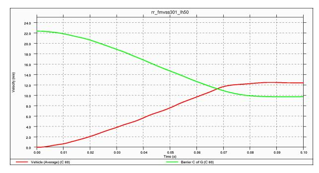
Figure 4.5.4.5.f shows the vehicle & barrier velocities.
