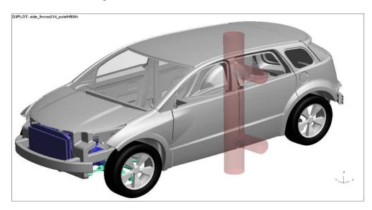
*Figure 4.5.4.3.a: 20-mph, 75-degree side-pole impact -- front (50th percentile male) model setup*
