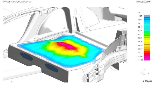
*Figure 4.3.5.2.b: Displacement at lower seatbelt anchorages (@0.2 s)*
