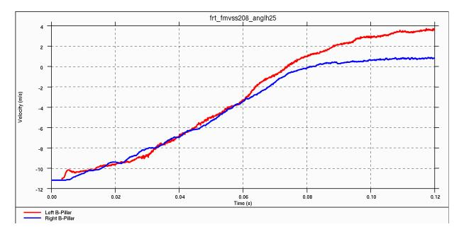
*Figure 4.3.3.d: Vehicle velocity during 30°, left-side frontal impact - time to 0 velocity* (TTZ) = 76 ms
