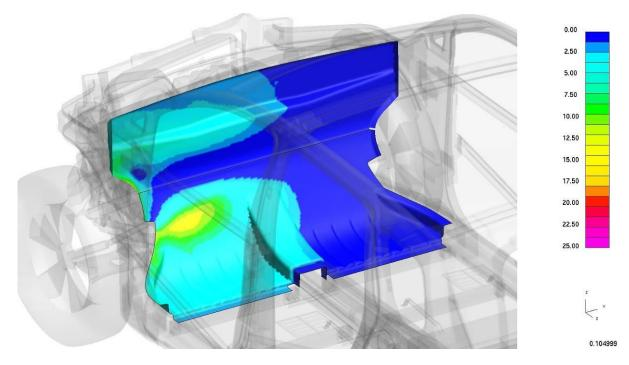
*Figure 4.3.3.f: CAE dash intrusion analysis after 30°, left-side frontal impact*
