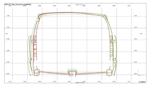
Figure 4.5.4.2.f shows the intrusion levels at the centerline of the B pillar.
