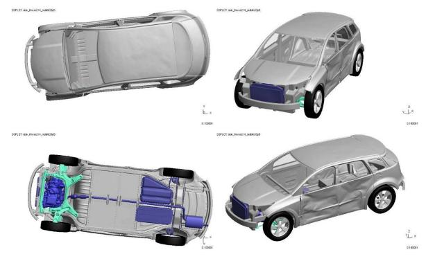
Figure 4.5.4.1.c: Vehicle Deformation (barrier not shown)
