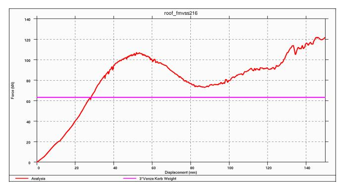
Figure 4.5.4.4.e: Roof Displacement vs. Applied Force – 3 times Venza Weight
