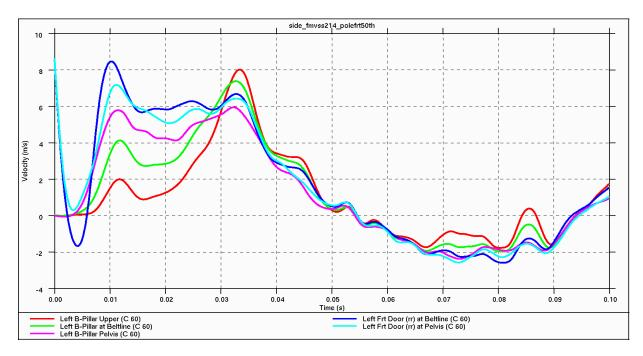
*Figure 4.5.4.3.d: Intrusion Velocities (B-Pillar & Front Door) after 20-mph, 75-degree side-pole impact -- front (50<sup>th</sup> percentile male)*
