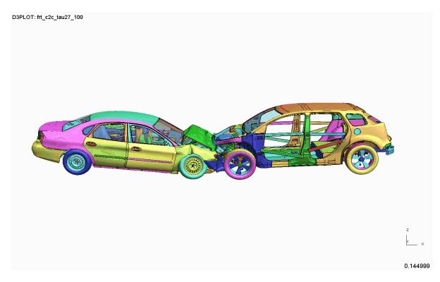
Figure 4.4.9.d: Phase 2 HD vehicle to Ford Taurus crash simulation result – side view
