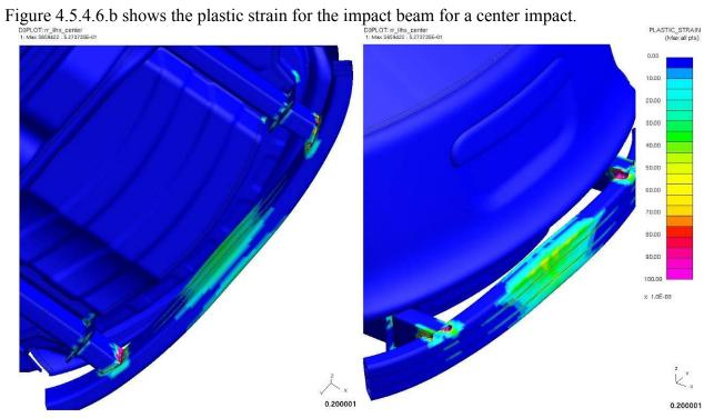
Figure 4.5.4.6.b: IIHS low-speed impact element plastic strains ('full')
