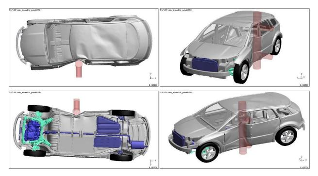
Figures 4.5.4.2.b and 4.5.4.2.c show the vehicle deformation following the pole strike.
