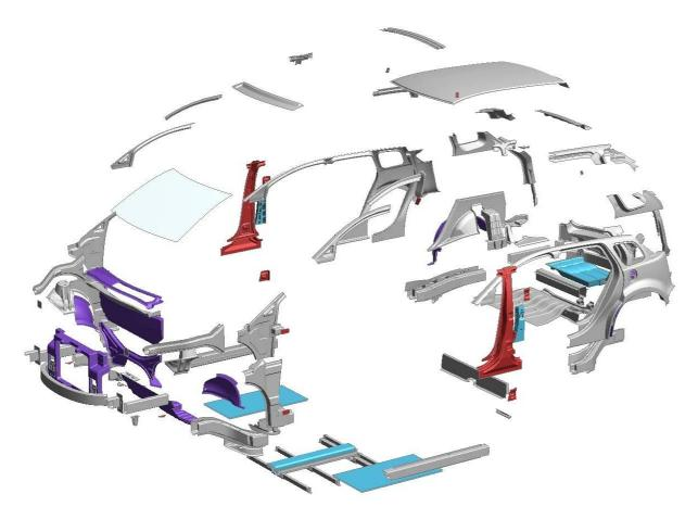
Figure 4.2.3.d: Body-in-white Material Usage Exploded View
