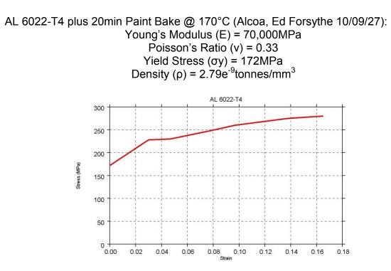
Figure 4.2.2.2.b: 6022 aluminum stress-strain curve
