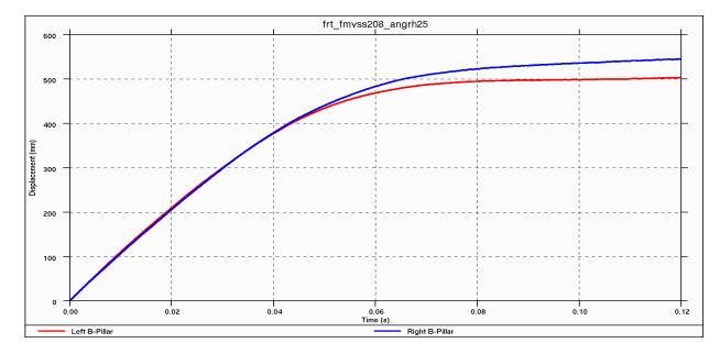
*Figure 4.3.4.e: Vehicle displacement during 30°, right-side frontal impact - maximum dynamic crush 524 mm*
