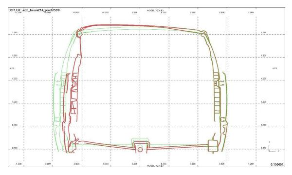
Figure 4.5.4.3.g: Section through B-Pillar, x = 2842 after 20-mph, 75-degree side-pole impact -- front (50<sup>th</sup> percentile male)
