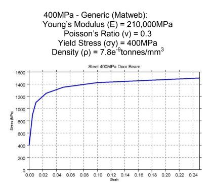
Figure 4.2.2.1.b: Steel stress-strain curve at 400 MPa
