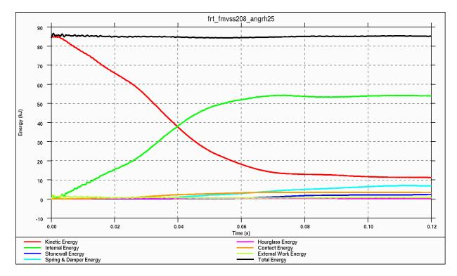
*Figure 4.3.4.i: Energy balance for 30°, right-side frontal impact*
