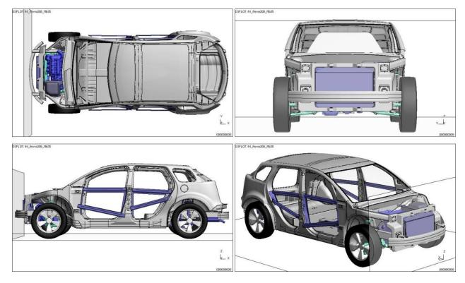
Figure 4.2.5.1.a: Rigid, deformable wall crash-test model setup
