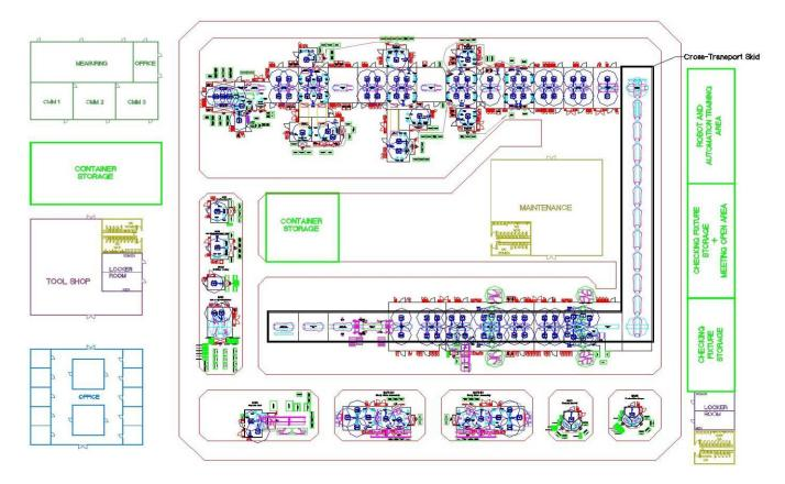
Figure 2.7.at: Overall body shop assembly layout
