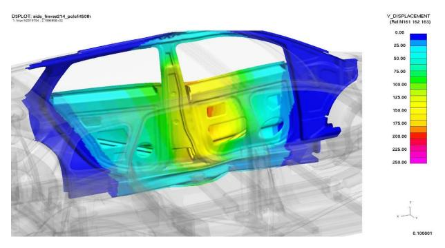
Figure 4.5.4.3.f: Intrusion levels on struckside after 20-mph, 75-degree side-pole impact -- front ( $50^{th}$  percentile male)
