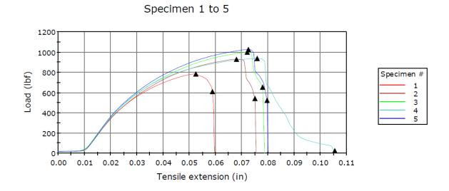
Figure 4.2.4.b: Henkel & Kawasaki lap-shear tests
