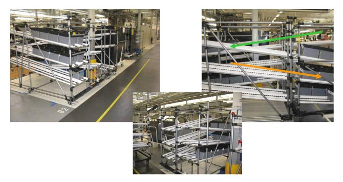
Figure 5.1.b: Shoot technology used to transport small parts
