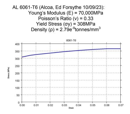
Figure 4.2.2.2.c: 6061 aluminum stress-strain curve
