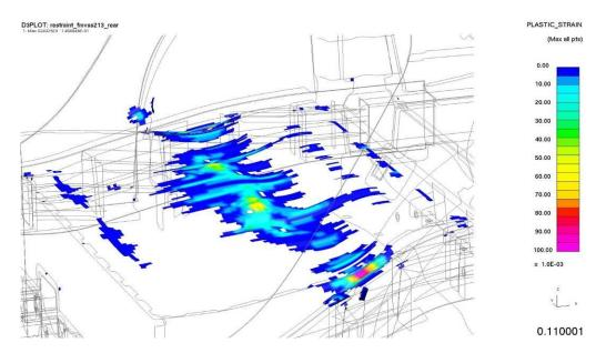
Figure 4.3.6.a: Child-restraint, lower anchorage plastic strain
