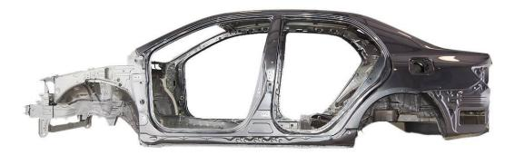
*Figure 4.5.8.1.7.b: Toyota Corolla body-in-white structure*
