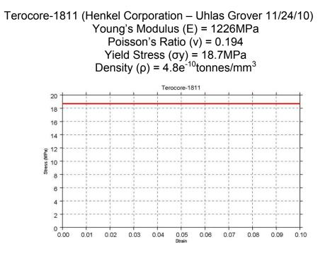
Figure 4.2.2.5.a: 1811 Terocore stress-strain curve
