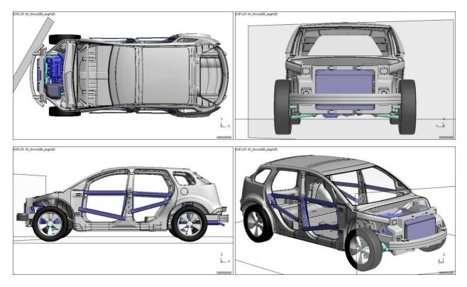
*Figure 4.2.5.4.a: 30°, right-side barrier crash-test model setup*
