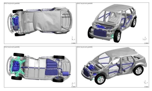
Figure 4.3.8.b: Vehicle deformation after 75°, side, pole impact (pole blanked) – 5th percentile female
