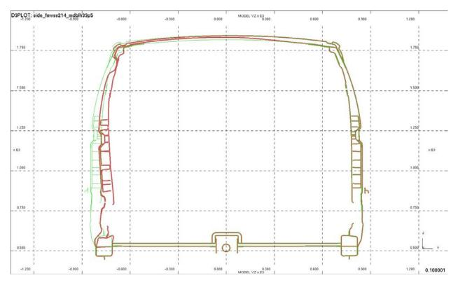
*Figure 4.3.7.f: B-pillar intrusion profile after crabbed barrier impact, x=2842*
