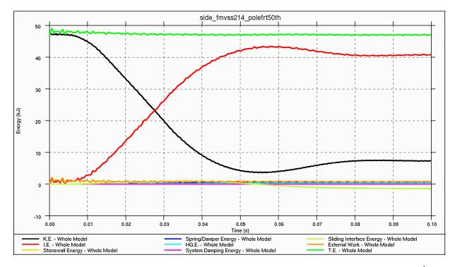
*Figure 4.5.4.3.i: Energy Balance for 20-mph, 75-degree side-pole impact -- front (50<sup>th</sup> percentile male)*
