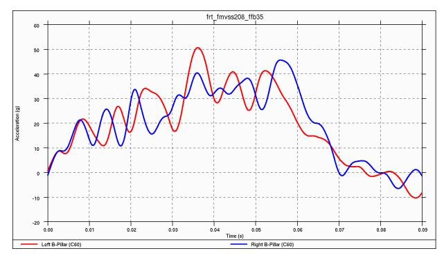
Figure 4.3.1.b: Vehicle acceleration pulse during frontal impact
