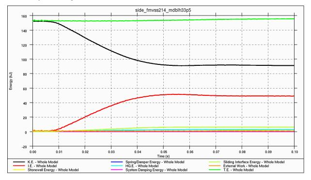
Figure 4.3.7.i: Energy balance for crabbed barrier impact
