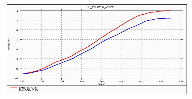
*Figure 4.3.2.e: Vehicle velocity after 40-percent overlap frontal impact - time to zero (TTZ)* = 0.117 s
