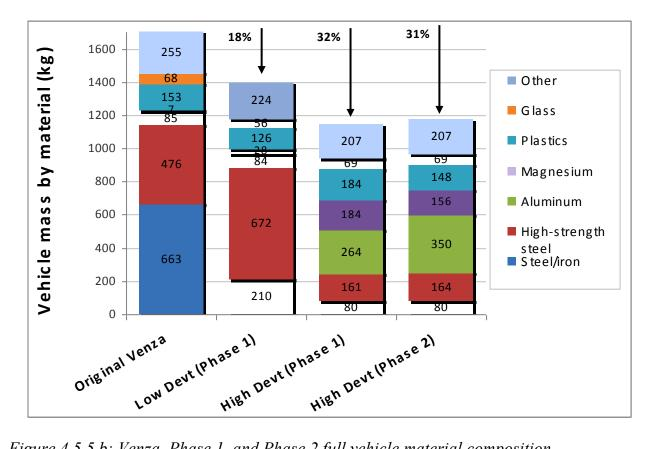
Figure 4.5.5.b below shows the total vehicle material utilization by mass for the baseline, Phase 1, and Phase 2 models.
