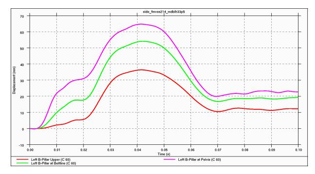
Figure 4.5.4.1.f: Relative Intrusion Displacements (B-pillar)
