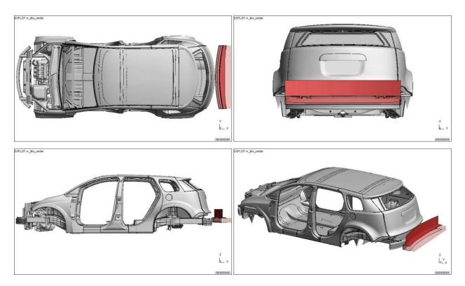
Figure 4.5.4.6.a: Low-speed IIHS impact model setup ('full')
