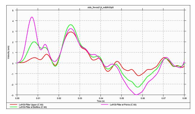
Figure 4.5.4.1.e: Relative Intrusion Velocities (B-pillar)
