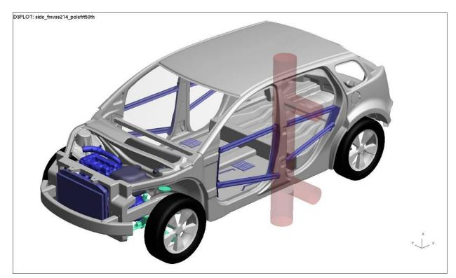
Figure 4.2.5.9.a: Side-pole impact test model setup
