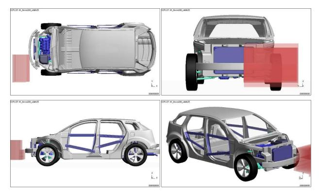
Figure 4.2.5.2a: 40-percent barrier overlap crash-test model setup
