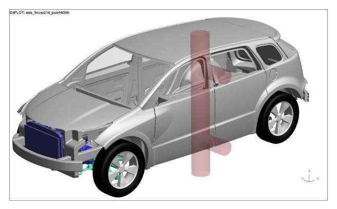
*Figure 4.5.4.2.a: 20-mph, 75-degree side-pole impact -- front (5th percentile female) model setup*
