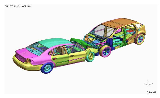
*Figure 4.4.9.c: Phase 2 HD vehicle to Ford Taurus crash simulation result – three-quarter view*
