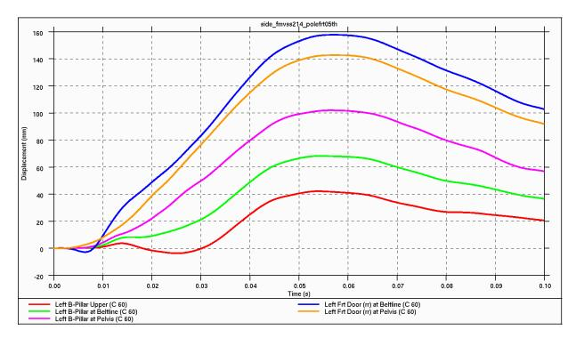
Figure 4.5.4.2.e: Intrusion Displacements (B-Pillar& Front Door)
