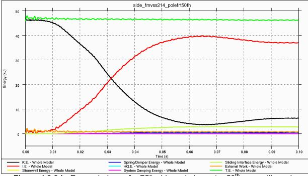
Figure 4.3.9.h: Energy balance for 75°, side, pole impact – 50<sup>th</sup> percentile male
