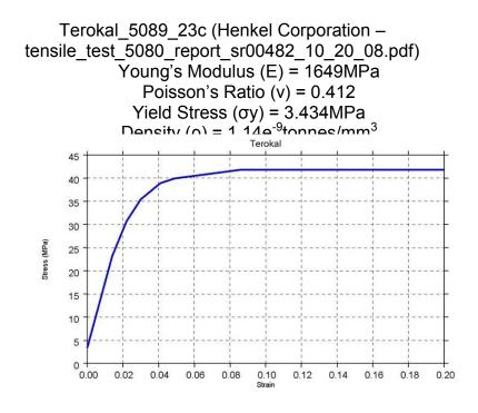
Figure 4.2.2.5.b: Terokal stress-strain curve
