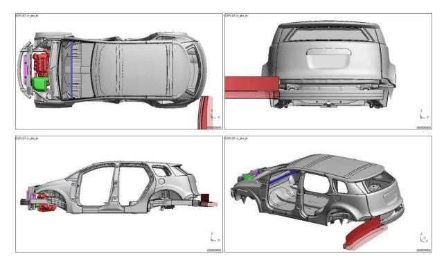
Figure 4.5.4.6.c: IIHS low-speed impact model setup ('offset')
