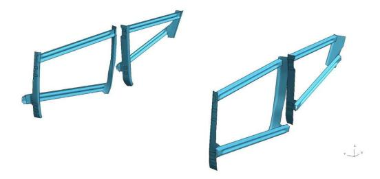
Figure 4.2.1.2.a: Simulated door beams
