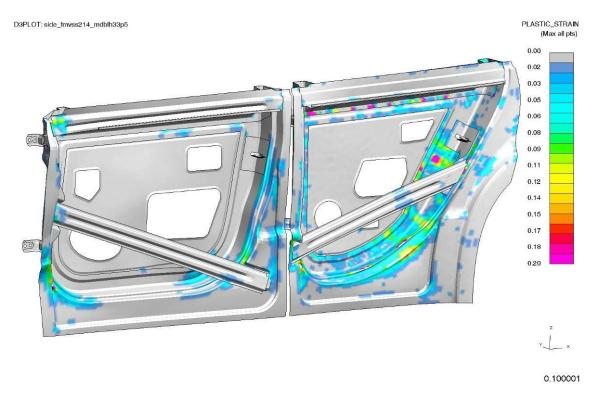
Figure 4.5.4.1.j shows the plastic strain for the struck side of the car.
