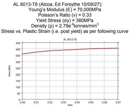
Figure 4.2.2.2.a: 6013 aluminum stress-strain curve
