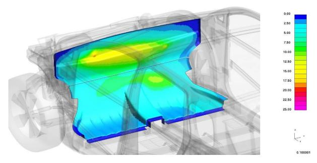
Figure 4.3.1.g: CAE dash intrusion analysis after frontal impact
