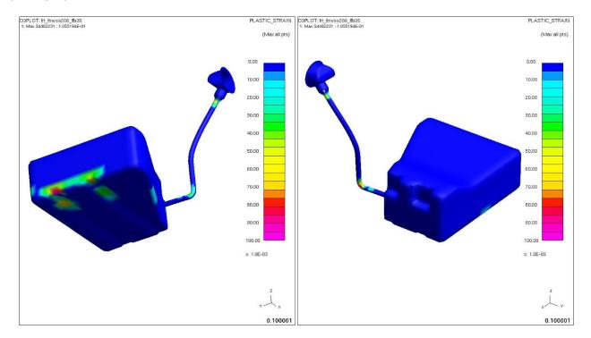
Figure 4.3.1.h: Fuel tank plastic strain after impact
