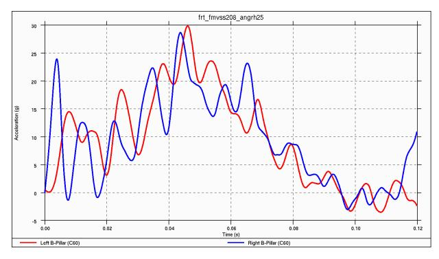
Figure 4.3.4.b: Vehicle acceleration pulse during 30°, right-side frontal impact
