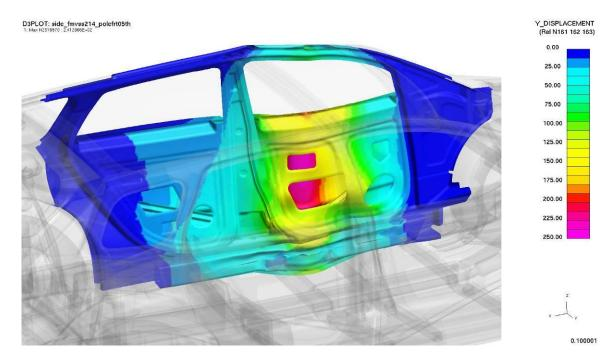
Figure 4.5.4.2.g: Intrusion levels on struck side
