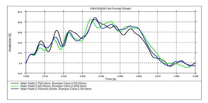
Figure 4.3.1.e: Vehicle acceleration during frontal impact
