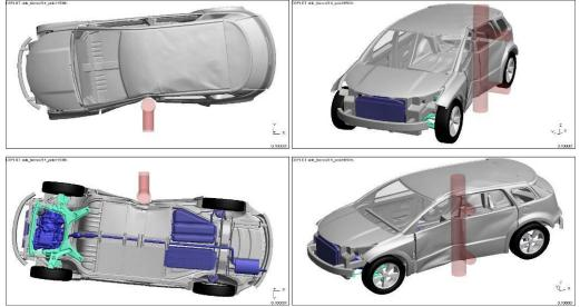
Figure 4.5.4.3.b: Vehicle Deformation (0.1s) after impact
