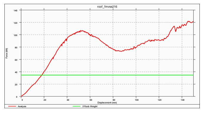
Figures 4.5.4.4.d and 4.5.4.4.e show the roof deformation relative to the FMVSS 216 requirement.
