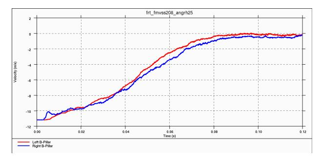
Figure 4.3.4.d: Vehicle velocity during 30°, right-side frontal impact
