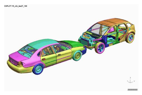
*Figure 4.4.9.a: Phase 2 HD vehicle to Ford Taurus crash simulation setup – three-quarter view*
