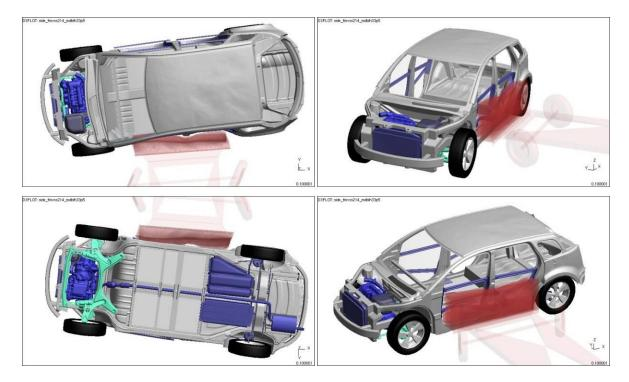
Figure 4.3.7.a: Vehicle deformation (0.1 s) after crabbed barrier impact
