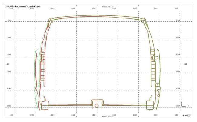
*Figure 4.5.4.1.h: B-Pillar Intrusion profile x=2842*
