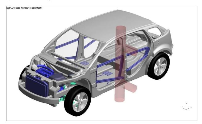
Figure 4.2.5.8.a: Side-pole impact test model setup
