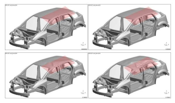
Figure 4.5.4.4.b shows the roof deformation for a series of increasing platen displacements.
