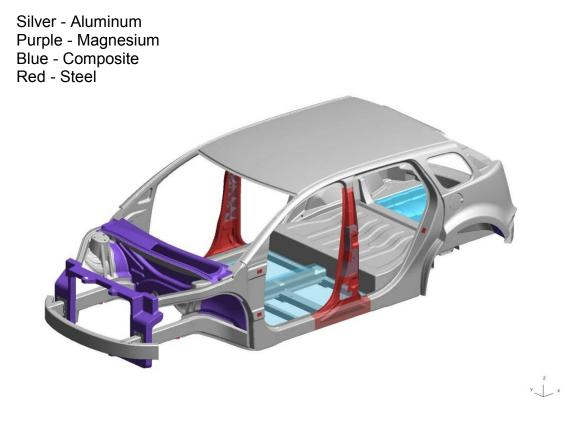
*Figure 4.2.3.a: Body-in-white material usage front three-quarter view*
