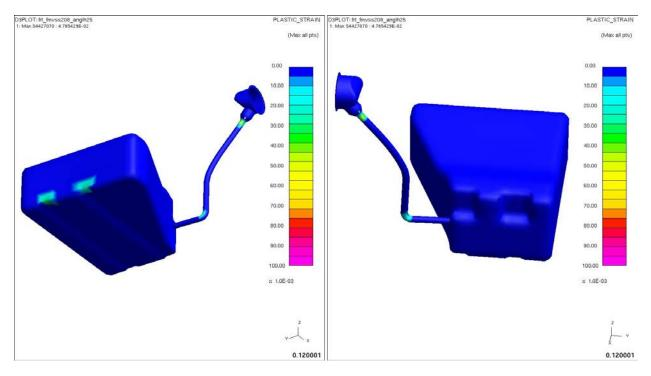
*Figure 4.3.3.g: Fuel tank plastic strain after 30°, left-side frontal impact*
