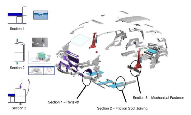
Figure 4.2.4.a: Typical Joint Sections
