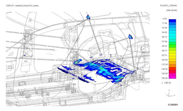
*Figure 4.3.5.2.a: Rear seatbelt anchorage plastic strain (@ 0.2 s)*
