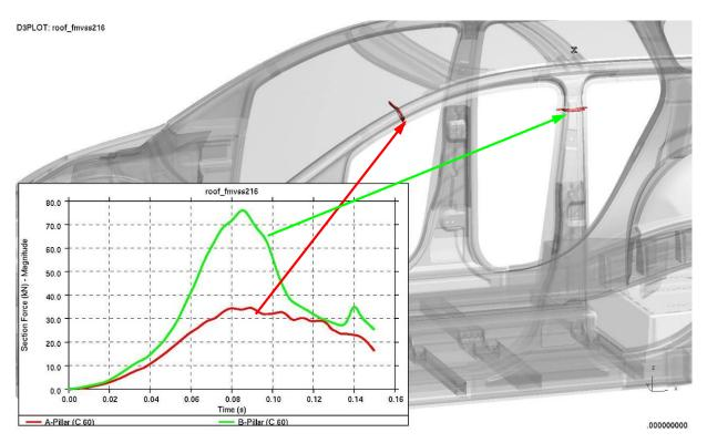
Figure 4.5.4.4.1.a: Resultant force magnitude in A & B-Pillars from roof crush test
