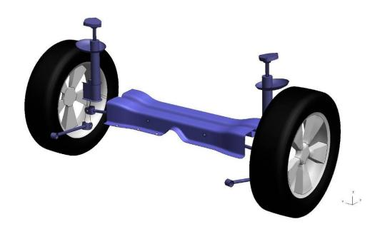
Figure 4.2.1.4.a: Rear sub-frame and suspension
