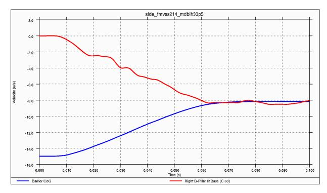
Figure 4.3.7.c: Global vehicle and barrier velocities for crabbed barrier impact
