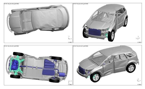
Figure 4.5.4.3.c: Vehicle Deformation (Pole Blanked)
