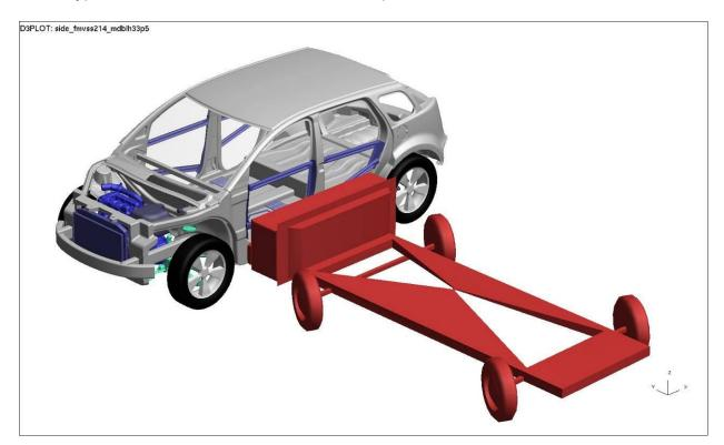
Figure 4.2.5.7.a: Crabbed barrier test model setup
