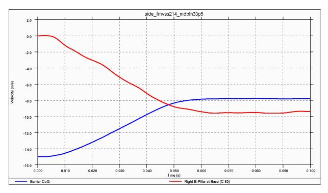
Figure 4.5.4.1.d: Global Vehicle and Barrier Velocities
