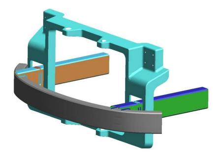
*Figure 4.3.1.i: Main energy absorbing frontal body structure*
