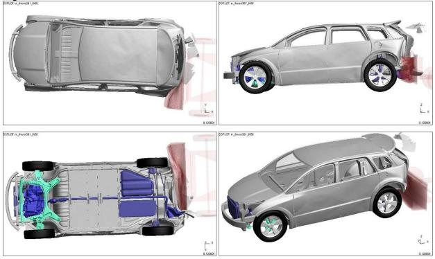
Figures 4.5.4.5.b and 4.5.4.5.c show the vehicle deformation.
