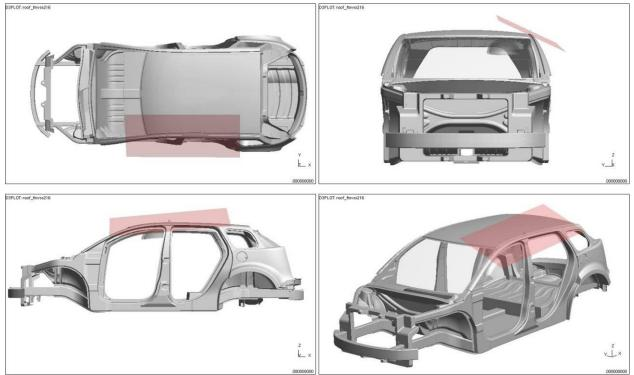
Figure 4.2.5.10.a: Roof crush test model setup
