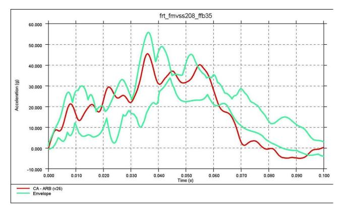
*Figure 4.3.2.1: Comparison of production vehicle envelope and Phase 2 HD crash accelerations*
