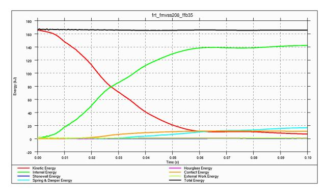
Figure 4.3.1.j: Energy balance for frontal impact
