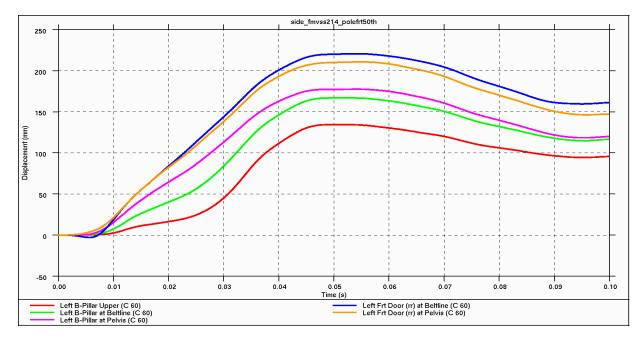
*Figure 4.5.4.3.e: Intrusion Displacements (B-Pillar & Front Door) after 20-mph, 75-degree side-pole impact -- front (50<sup>th</sup> percentile male)*
