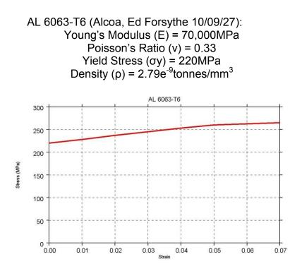
Figure 4.2.2.2.d: 6063 aluminum stress-strain curve
