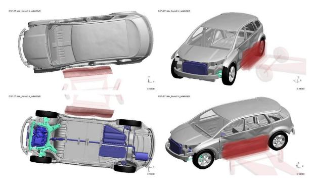
Figures 4.5.4.1.b and 4.5.4.1.c below show the vehicle deformation following impact.
