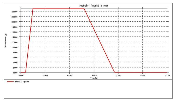
Figure 4.2.5.6.a: Acceleration pulse applied to child-restraint model
