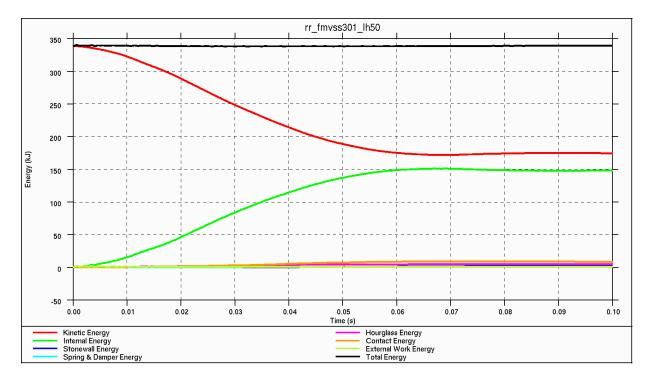
Figure 4.5.4.5.h shows the energy balance verifying that the overall energy is held constant.
