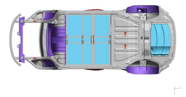
Figure 4.2.3.c: Body-in-white material usage underbody view
