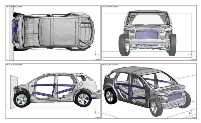
Figure 4.3.1.a: Vehicle deformation (t=0.1 s) after frontal impact
