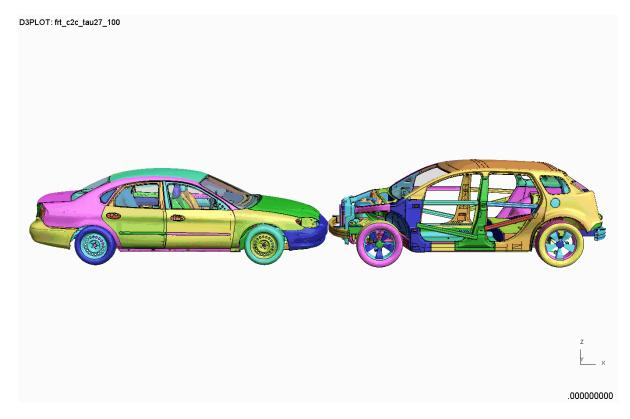
*Figure 4.4.9.b: Phase 2 HD vehicle to Ford Taurus crash simulation setup – side view*
