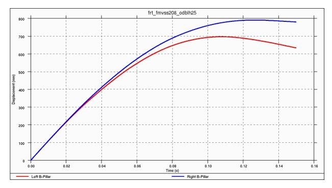
Figure 4.3.2.f: Vehicle displacement after 40-percent overlap frontal impact
