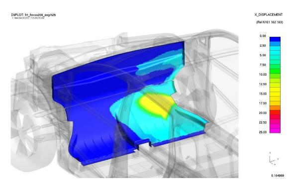
Figure 4.3.4.f: CAE dash intrusion analysis after 30°, right-side frontal impact
