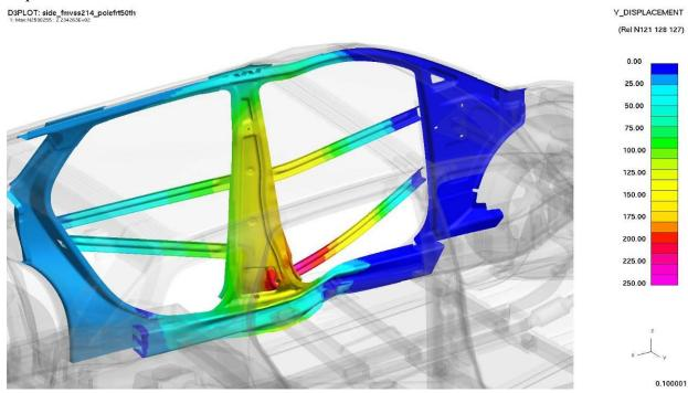
Figure 4.3.9.e: Intrusion levels after 75°, side, pole impact on struck side  $-50^{th}$  percentile male
