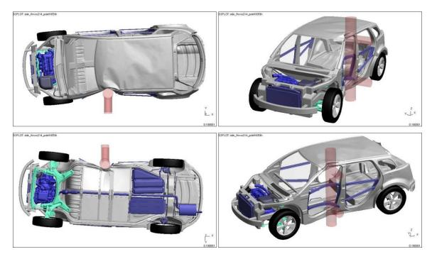
Figure 4.3.8.a: Vehicle deformation (0.1 s) after 75°, side, pole impact – 5th percentile female
