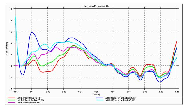
Figures 4.5.4.2.d and 4.5.4.2.e show the intrusion velocities and displacements for the B pillar and front door.
