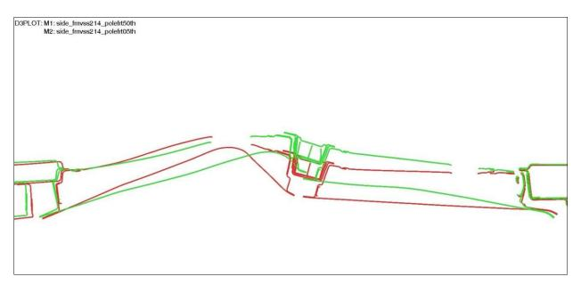
*Figure 4.5.4.3.1.a:* 5<sup>th</sup> percentile female vs. 50<sup>th</sup> percentile male front door intrusion comparison
