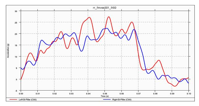
Figure 4.5.4.5.e: Vehicle Acceleration Pulse during rear impact
