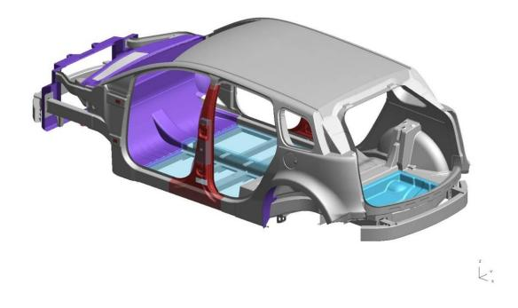
*Figure 4.2.3.b: Body-in-white material usage rear three-quarter view*
