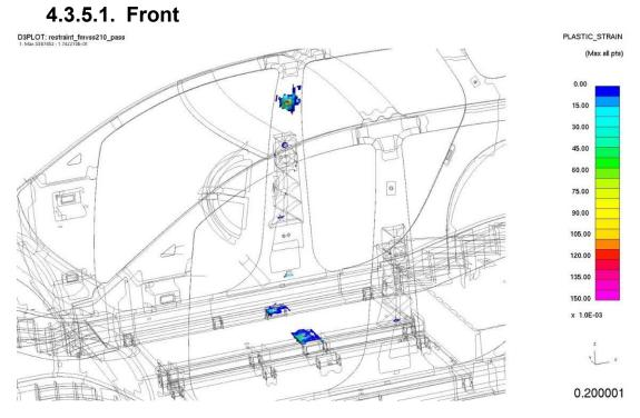
*Figure 4.3.5.1.a: Seatbelt anchorage plastic strains (@ 0.2 s)*
