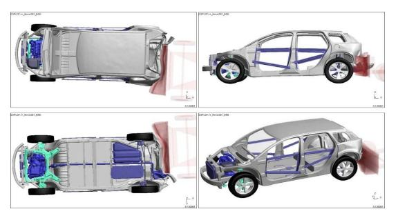
*Figure 4.3.11.a: Vehicle deformation (t=0.12 s) after rear deformable barrier impact*
