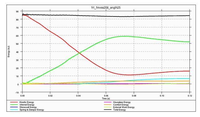
Figure 4.3.3.i: Energy balance for 30°, left-side frontal impact
