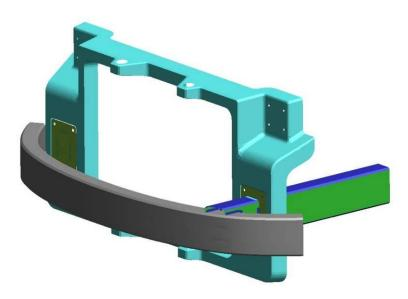
*Figure 4.3.2.i: Main energy absorbing body structure – 40-percent overlap frontal impact*
