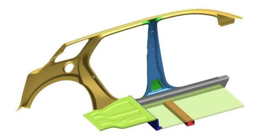
*Figure 4.3.9.g: Main energy absorbing body structure for 75°, side, pole impact*  $-50^{th}$  *percentile male*
