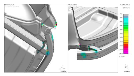
Figure 4.3.13.b: Rear plastic strains after low-speed rear impact ('offset impact')
