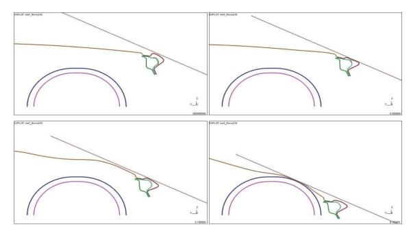
*Figure 4.5.4.4.c: Deformation in Relation to occupant head clearance zones (95<sup>th</sup>/99<sup>th</sup>) (a) 0/40/80/150mm of Platen Displacement*
