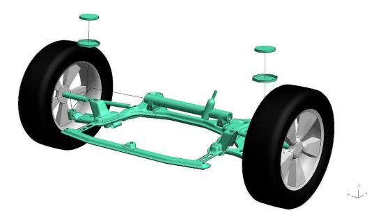
Figure 4.2.1.3.a: Front sub-frame and suspension
