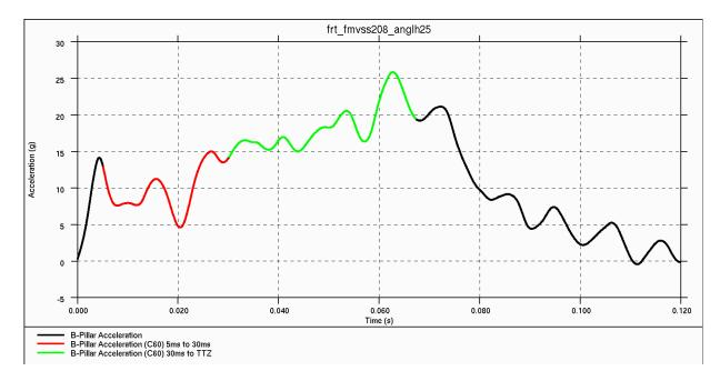
*Figure 4.3.3.c: Average vehicle acceleration pulse during 30°, left-side frontal barrier impact*
