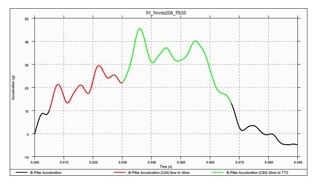
Figure 4.3.1.c: Average vehicle acceleration pulse during frontal impact
