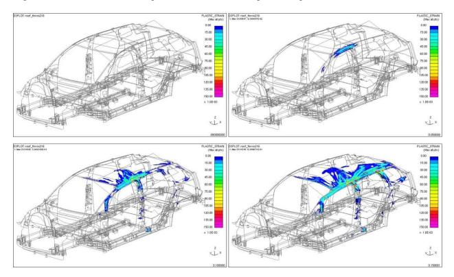
Figure 4.5.4.4.f shows the roof plastic strain relative to platen displacement.
