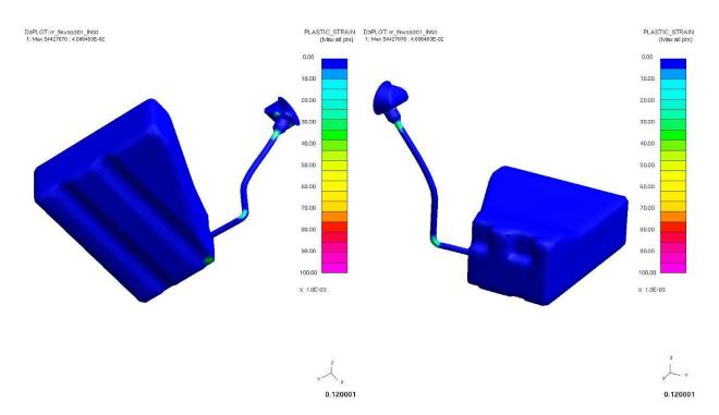
Figure 4.5.4.5.g: Fuel Tank Plastic Strains after rear impact
