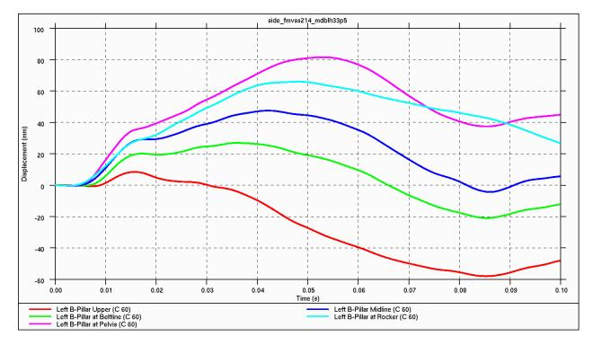
Figure 4.3.7.e: Relative intrusion displacements (B-pillar) during crabbed barrier impact
