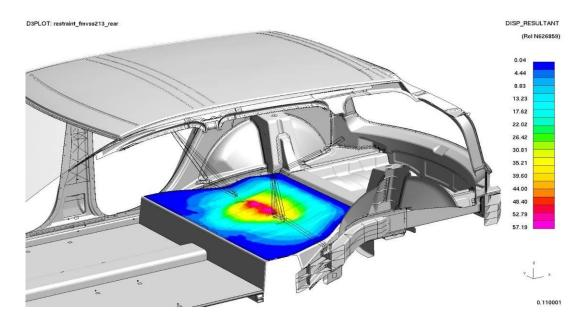
*Figure 4.3.6.b: Child-restraint seat pan displacements*
