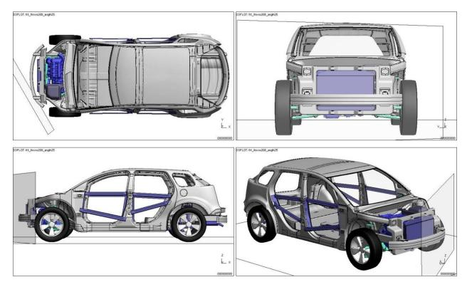
*Figure 4.2.5.3.a: 30°, left-side barrier crash-test model setup*
