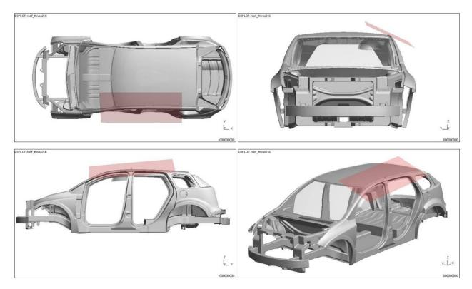
Figure 4.5.4.4.a: Roof crush model setup
