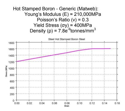
4.2.2.1.c: Hot-stamped, boron steel stress-strain curve
