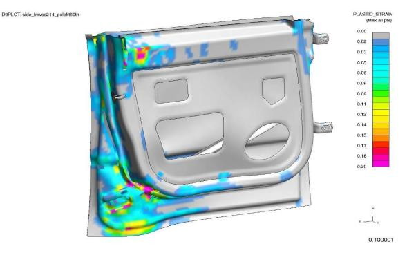
Figure 4.5.4.3.h: Plastic Strain in Front Door after 20-mph, 75-degree side-pole impact -- front ( $50^{th}$  percentile male)
