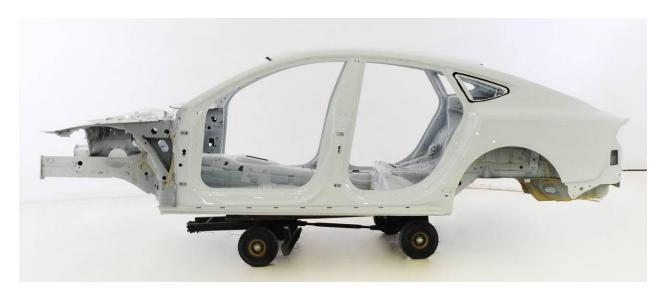
Figure 4.5.8.1.7.d: Audi A7 body-in-white-structure
