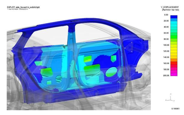
Figure 4.5.4.1.i: Intrusion levels on Struck-side
