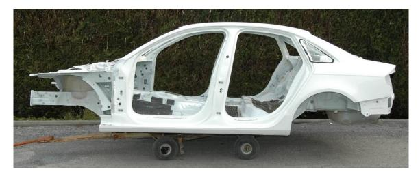
Figure 4.5.8.1.7.c: Audi A4 body-in-white structure
