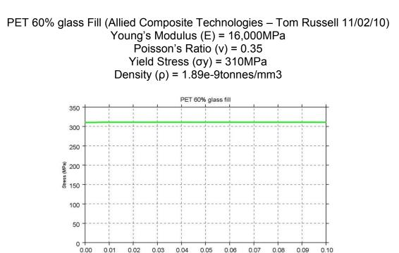
Figure 4.2.2.4.b: 60-percent glass-fiber PET stress-strain curve
