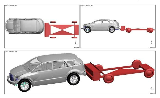
Figure 4.5.4.5.a: Rear Impact Model Set up
