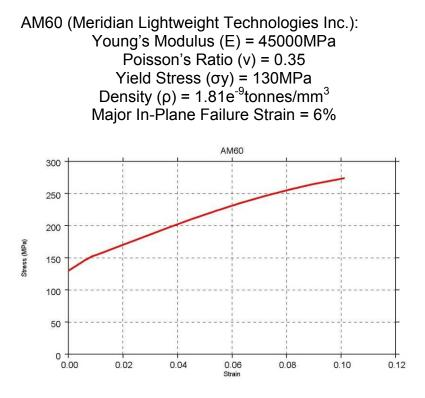
Figure 4.2.2.3.a: AM60 magnesium stress-strain curve
