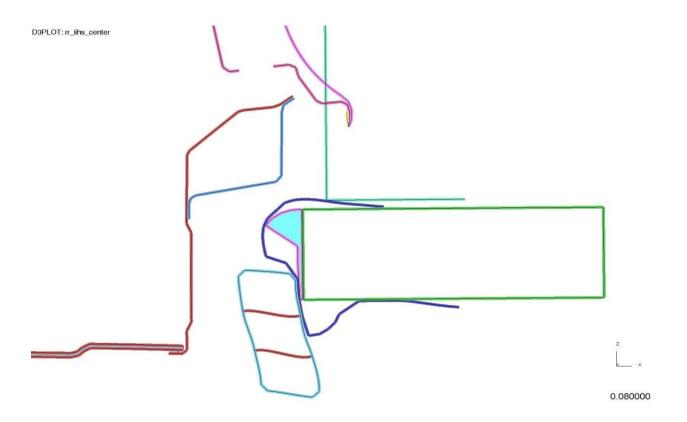
Figure 4.5.4.6.1.a: Maximum deflection showing barrier intrusion into tailgate
