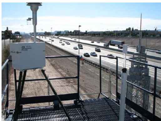
Part of an air monitoring station along the I-15 highway corridor in Las Vegas, Nevada, used in the near-road monitoring project the EPA conducted with the U.S. Department of Transportation's Federal Highway Administration. (EPA photo)
