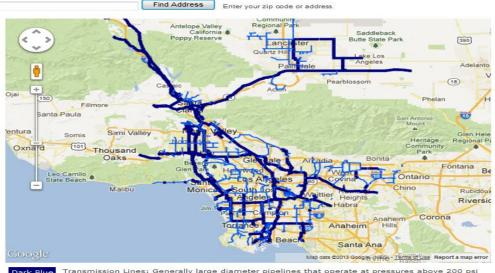
Transmission Lines: Generally large diameter pipelines that operate at pressures above 200 psi and transport gas from supply points to the gas distribution system.
