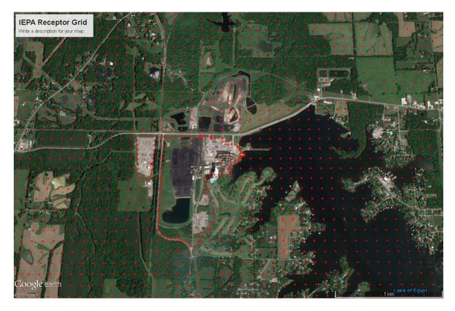
In this figure, red dots are used to indicate the locations of receptors in Illinois' modeling. The Marion power plant is in the center of this figure, and Lake Egypt Road runs east-west through the center of this figure. Thus this figure illustrates that Illinois used a regular grid of receptors in SIPC's property north of Lake Egypt Road, northeast of the plant.
