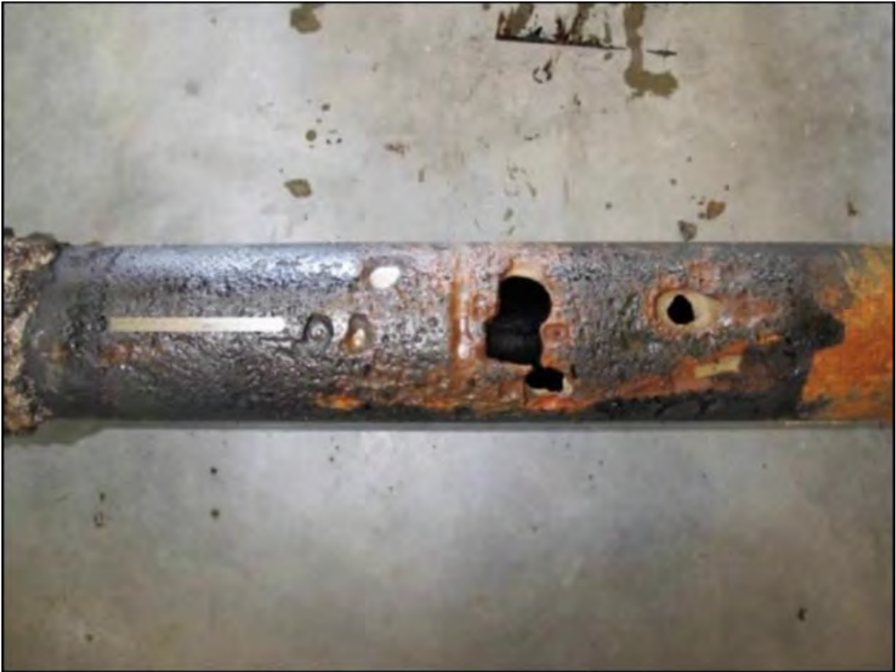
Figure 5. Large holes and corrosion damage on the top of the 6-inch-diameter water pipe
